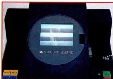
**Step 8:** Once the automatic process has been initiated, using a built-in camera and image processor, the machine positions the fibers, inspects the prepared ends, cleans them, and aligns the fiber cores in
