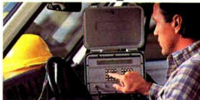
document leaks as weak as 10  $\mu\text{V}/\text{m}$ , with field strength measurement at frequencies from 50 to 550 MHz.
