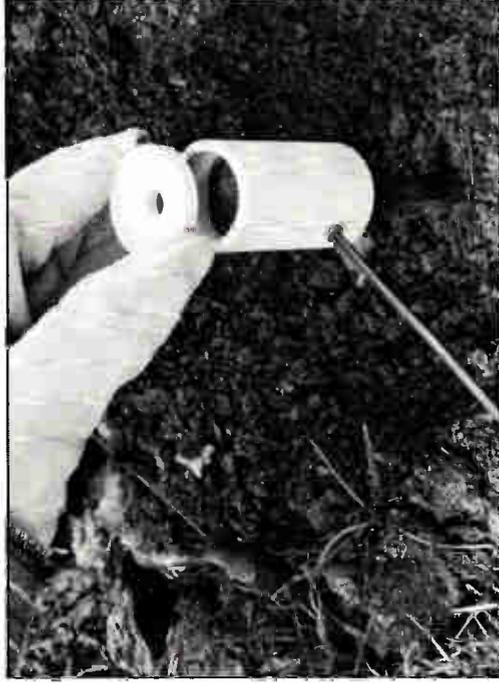
**Photo 6:** Place the cover on top of the mold.
