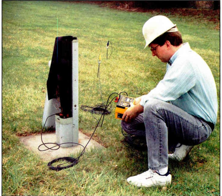
A technician checks grounds using a ground tester.
