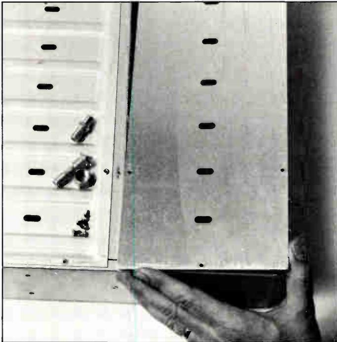
Step 15: After new connectors, jumpers and other components have been replaced, install the rear compartment cover.
