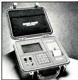
Model 1210 Universal TDR, Cable Fault Locator
