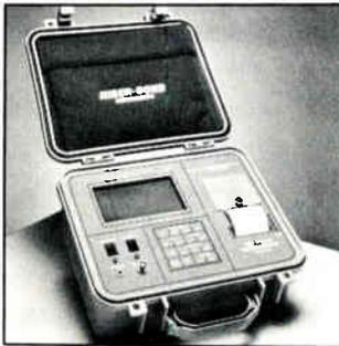
Model 1210 Universal TDR, Cable Fault Locator
