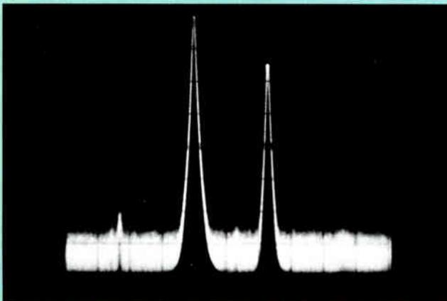
Figure 3: In-channel frequency response measured with Sin X/X test signal
