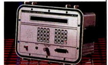
will measure the leakage and provide the correct and convenient reading in  $\mu\text{V}/\text{m}$ .
