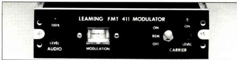
Each FMT411F modulator transmits one program audio channel. The FMT411F transmits the program material on any specified frequency between 4.5 & 10 MHz, 52 & 88 MHz or 88 & 126 MHz. Audio bandwidths of 3.4 kHz, 7.5 kHz, 10 kHz, or 15 kHz are available. Typical uses for the FMT411F include modulation of an audio signal to 4.5 MHz for transmission via fiber or microwave.
