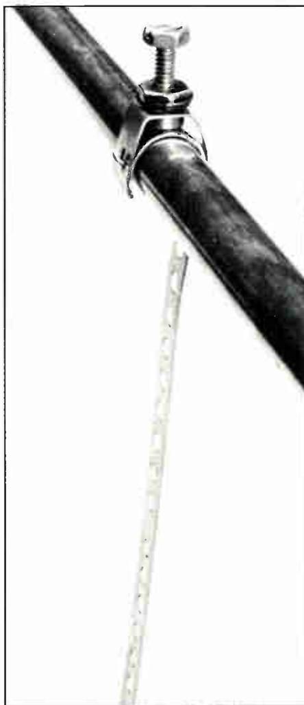
**Step 2:** Remove any corrosion or paint down to bare metal to ensure a clean surface that will provide a good ground connection. (Note: Do not remove the zinc coating on galvanized surfaces!) Install the strap on the pipe so the "U" shaped portion of the strap clamps itself to the surface. On larger diameter pipes, it may be necessary to form the strap to fit.
