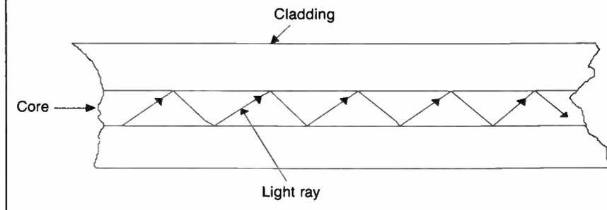
within an area outside the fiber known as the *acceptance cone* (Figure 3) will enter the core and be reflected down the fiber; all other light will be lost. The acceptance cone area is defined by the quantity called *numerical aperture* (NA), which is a measure of the light gathering ability of an optical fiber.
