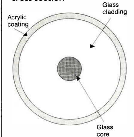
Core: 9  $\mu$ m - 100  $\mu$ m diameter
