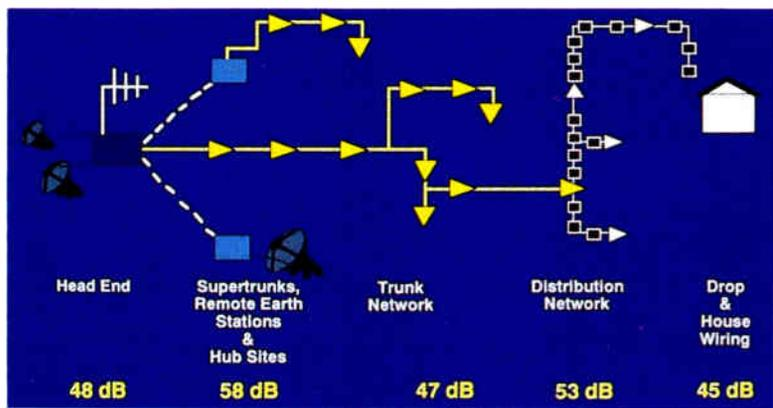
**Figure 2:** Conventional coax plant architecture
