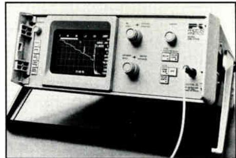
The OTDR gives a "picture" of the fiber along its length.
