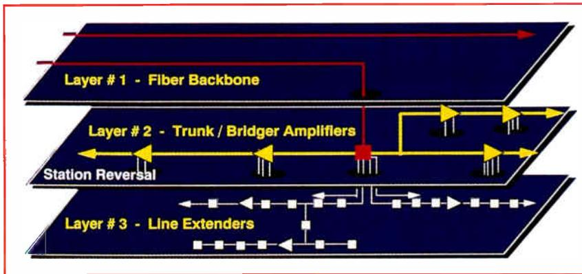
**Figure 4:** Fiber trunk and feeder architecture
