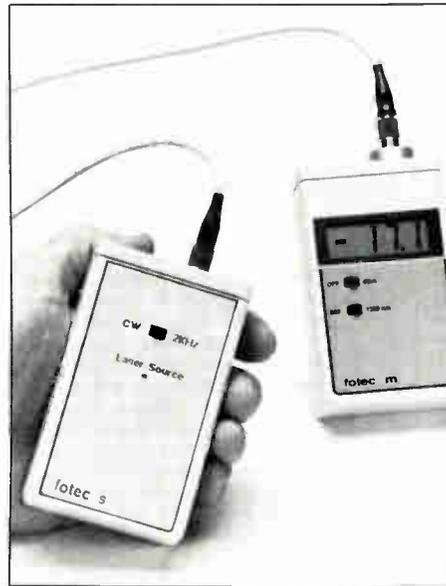
*The fiber-optic power meter is the most basic instrument. The laser source is used only for loss testing.*
