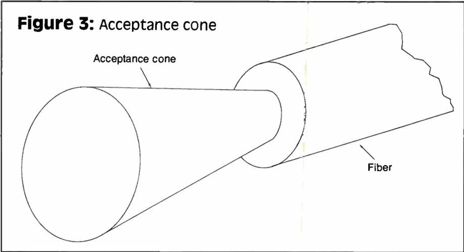
is 125 or 140  $\mu\text{m}$ . Multimode fibers allow multiple modes (light rays) to enter and travel through the core. Single-mode fibers have core sizes of 8.3, 8.7 and 9  $\mu\text{m}$ . Cladding diameter is 125  $\mu\text{m}$ . Single-mode fibers allow only one mode to enter and travel through the core.
