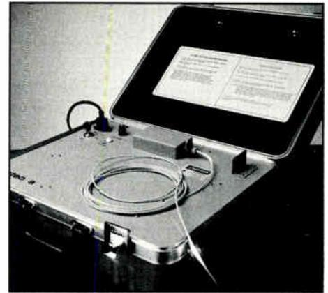
*The HeNe laser visual cable fault locator allows troubleshooting fiber-optic cables in the OTDR's "dead zone."*
