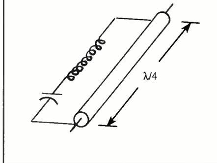
an inductor, and the open-circuited coax will take on the characteristics of a capacitor.
