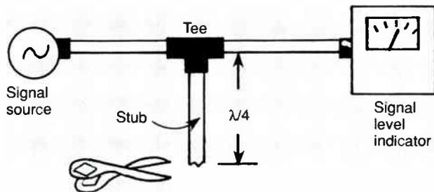
cable you use), the length of cable necessary to construct a quarter wavelength trap can be found with the following formula:
