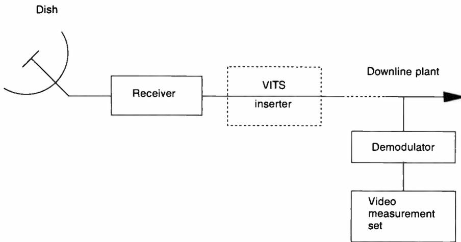
**Figure 4: Multiburst measurement of frequency response**
