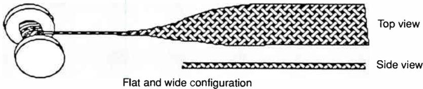
**Figure 12:** Wire mesh pulling grip
