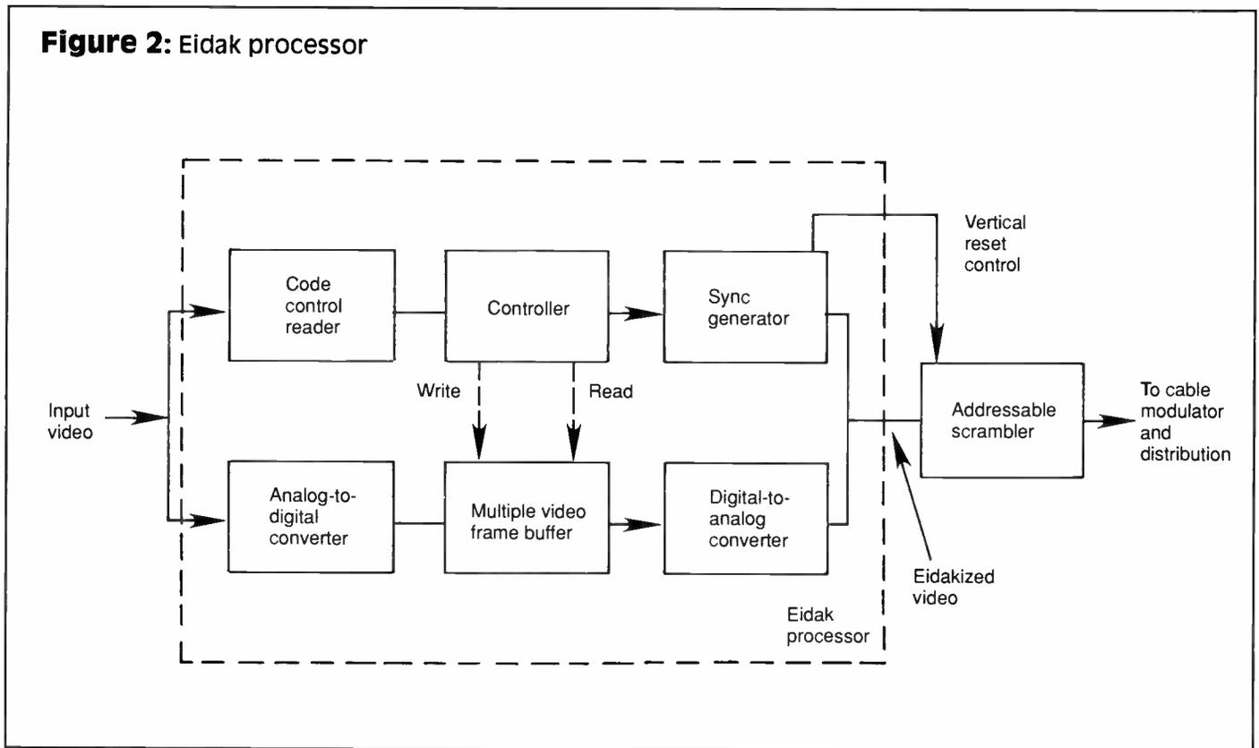
sync, some resynchronization must be provided for cable scramblers, which typically are dependent on precise VBI timing. For remote hub operations of scramblers, frame length data is encoded into the VBI and at the hub location an Eidak scrambler interface (ESI) converts the frame length information into resynchronization signals for the scrambler.
