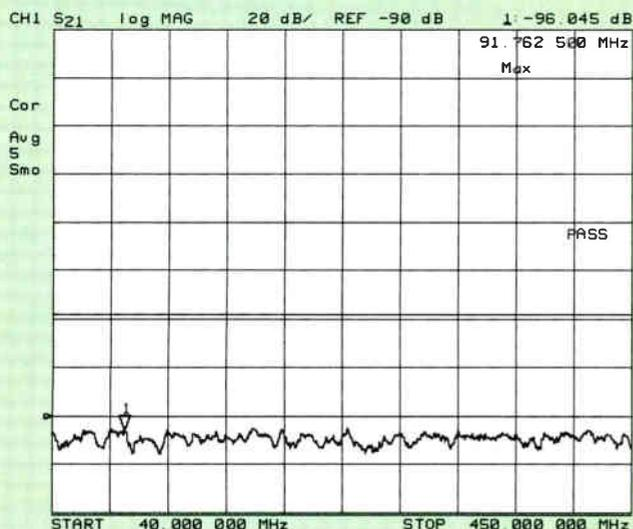
**Figure 2:** Typical RF shielding after temperature cycling from -40 to +60°C; again the shielding is at the noise floor of the measurement system
