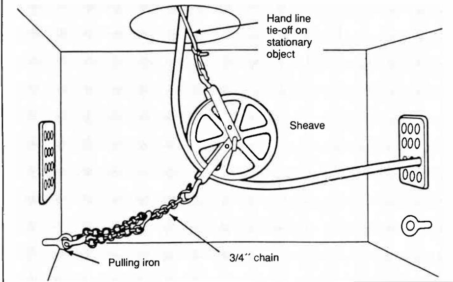
**Figure 17:** Cable reel setup
