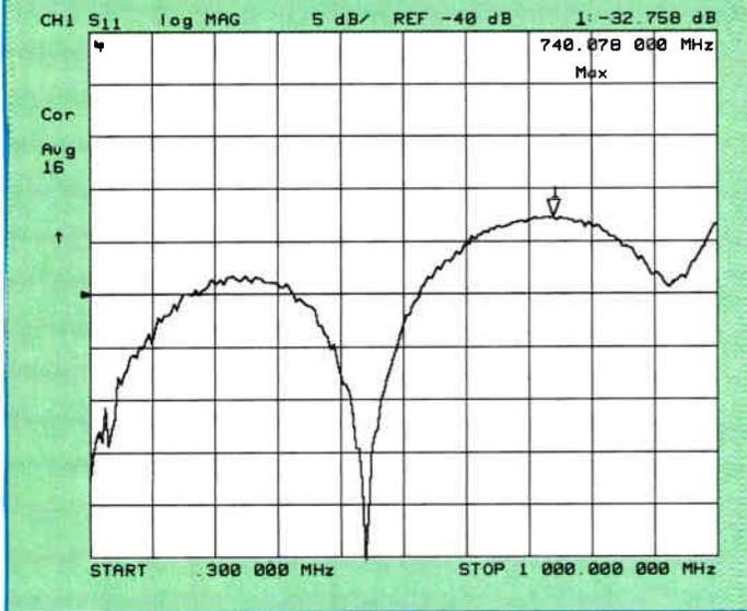
**Figure 4:** The .750 connectors had 30 dB or better return loss up to over 890 MHz (Marker 2) and 26.5 dB at 1 GHz
