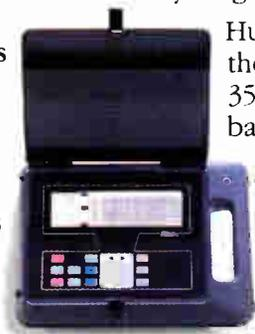
Hum and signal to noise are measured with the push of a button. You can store up to 35 test points in memory then call them back to the display screen, print out charts or graphs or download the information to a PC for further analysis. Delta Sweep option lets you compare real-time sweep data with readings from memory.
