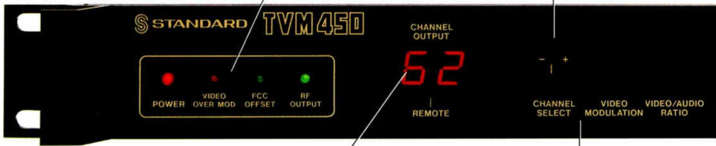
LED RF channel output indicator is displayed in numeric CATV channels. RF channel output mutes during channel selection or catastrophic RF failures.
