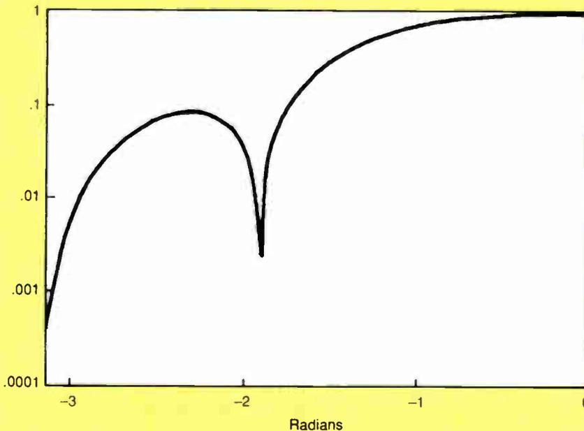
Stagger stacking may create more harm than good if the interfering signal arrives from a relative angle less than  $172^\circ$  or more than  $188^\circ$ . It is instructive to follow the development of the radiation pattern backlobes on Figures 4 through 6.
