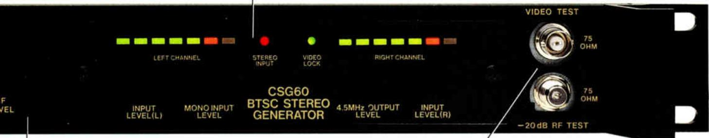
RF output purity, stability and video quality can be monitored with front panel video and RF output test ports.
