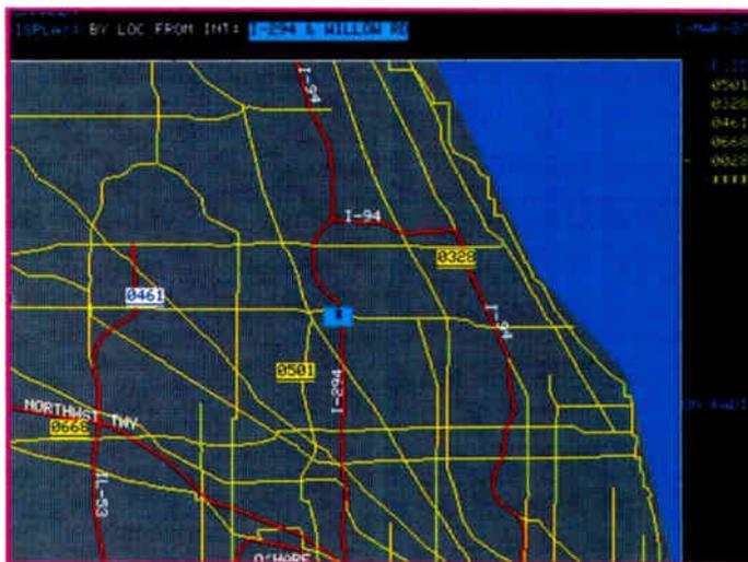
*Three levels of map displays can be viewed on the dispatcher's screen. The maximum view is 24x16 miles (above), the minimum is 6x4 miles (below).*
