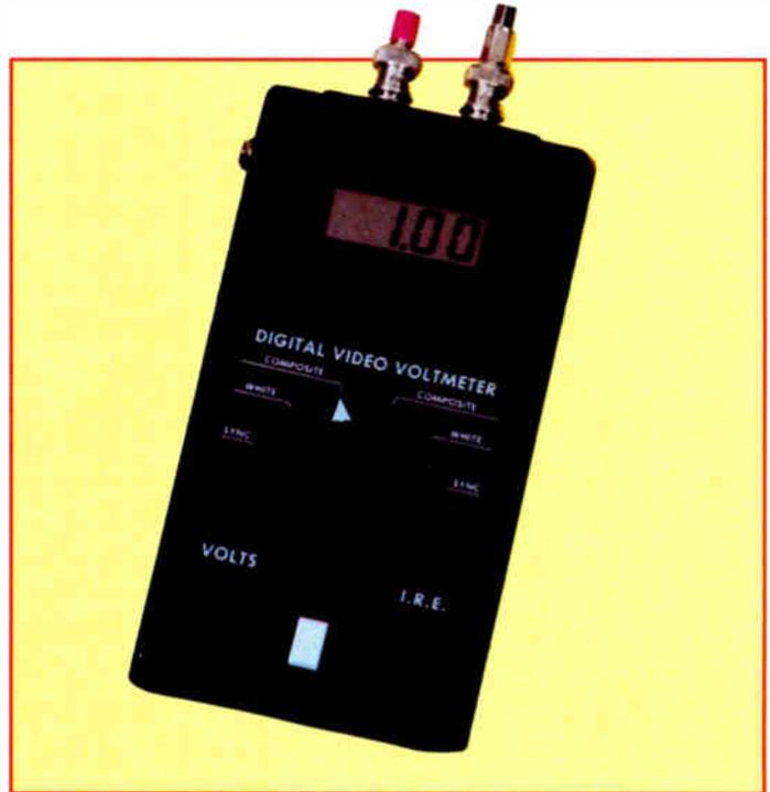
turned on with a front panel momentary contact rocker switch; an automatic off feature turns the VVM off after about one minute of use. The on time can be increased by pushing the switch again before the time-out occurs. Should internal battery voltage be too low to provide accurate readings, internal circuitry prevents the meter from operating when the on switch is pressed.
