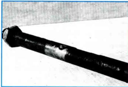
**Abnormal wear of hinge pin due to lack of regular lubrication.**
