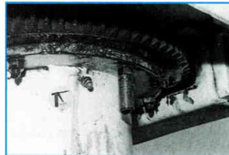
**Ring gear with enclosed box for worm gear and oil bath.**
