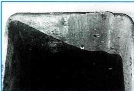
**Abnormal boom wear caused by worn pads.**
