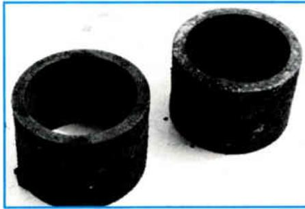
**Worn bushings, rusted from lack of grease.**
