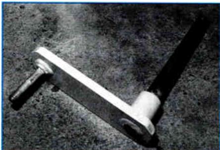
**New replacement hinge pin and leveling lever arm.**
