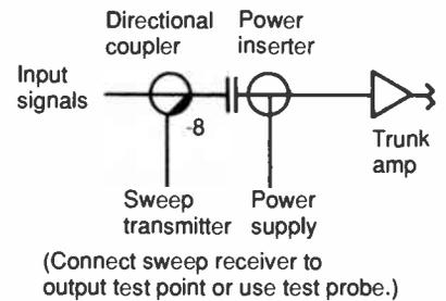
a system problem needing repair. Major response variations indicated system problems, while minor variations were compensated for using the adjustments on the amp module.
