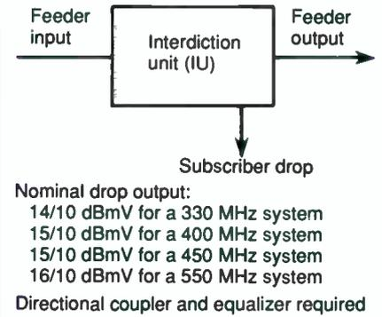
with interdiction parallels design with taps. With interdiction, the tap value is determined unit-by-unit with a plug-in directional coupler. Selection of the directional coupler is a similar process as selecting a face plate value in traditional tap systems.
