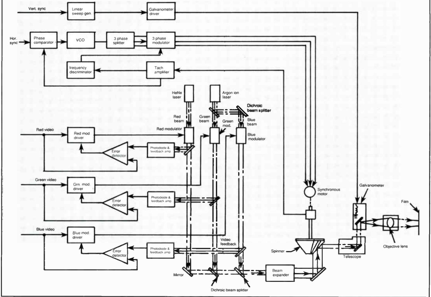
**Figure 5: Elements of the mechanically scanned laser-beam telecine**
