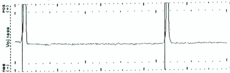
**Figure 2:** Waveform of 340 feet of .625 trunk cable with sheath damage in the middle
