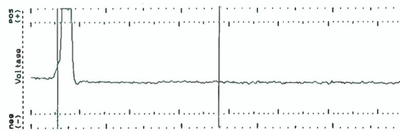
**Figure 3:** Waveform of 340 feet of .625 damaged trunk cable in saltwater
