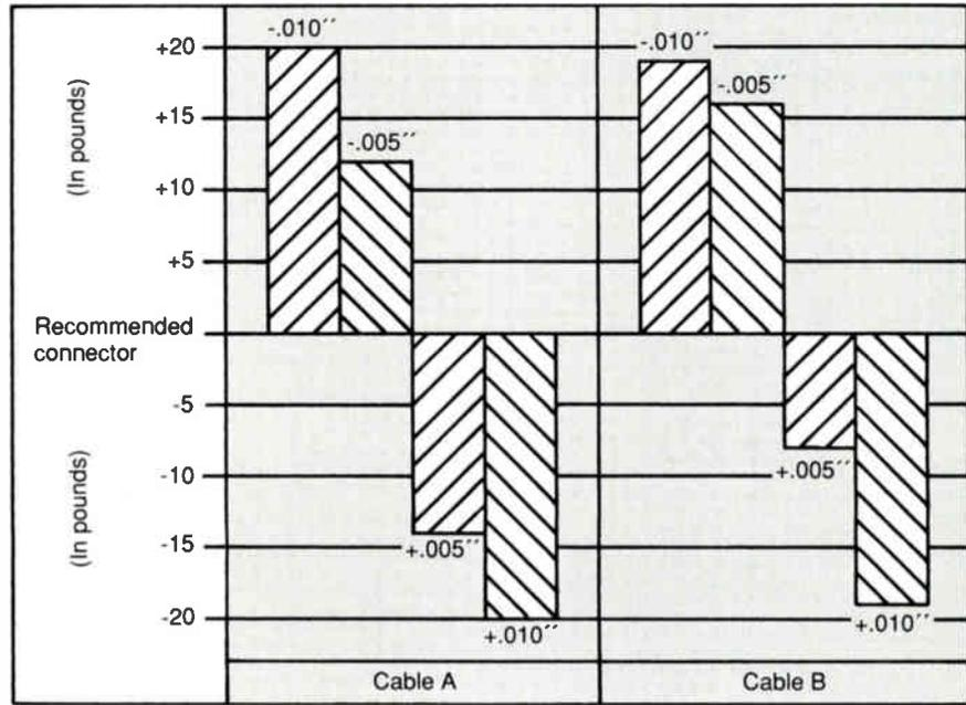
**Figure 3: Cable retention with different braid prep lengths (conventional connector)**
