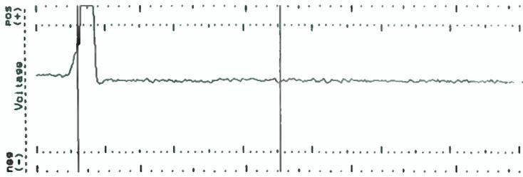
**Figure 5:** Waveform of 340 feet of .625 trunk cable with a wet, contaminated splice
