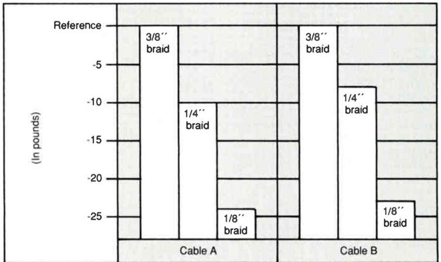
connector retention of the cable. A connector on a 53 percent braided cable should not be expected to have the same retention force as on a 95 percent braided cable. Figure 1 illustrates how the connector retention force varies with different braid coverage drop cables. These differences are mainly due the amount of metal in the outer shield.
