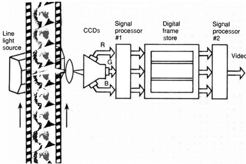
**Figure 7: Steps for production of successive-exposure master and color internegative in the Image Transform tape-to-film transfer system**
