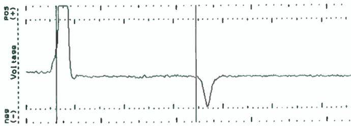
**Figure 6:** Waveform of a 400-foot cable containing three taps with values of 10, 12 and 17 dB at 100-foot intervals
