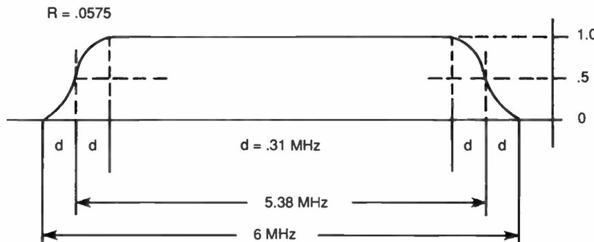
**Figure 10: DSC-HDTV/NTSC RF co-channels**
