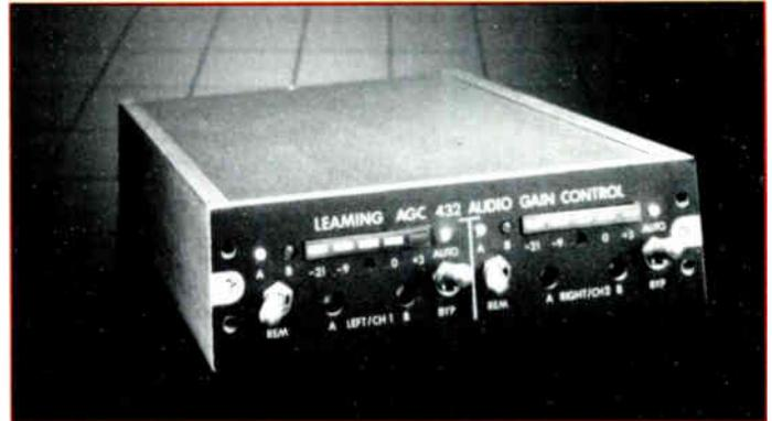
The AGC module itself is 1.6" H x 5.5" W x 10.5" D and is designed to be mounted in Leaming's PMU401 panel mount. The panel mount is 19" W x 1-3/4" H and will hold either three AGC modules or two modules and a PS420 power supply. Up to five AGC432s can be powered from the PS420. An external power supply also can be used; requirements are +24 volts DC @ 150 mA per module.
