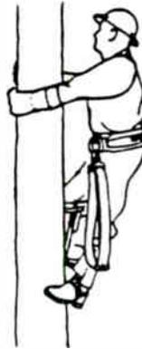
**Figure 12:** Releasing safety strap
