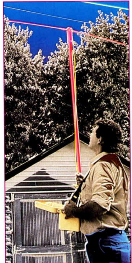
**A technician uses a dipole and meter to make a 10-foot measurement under overhead lines.**
