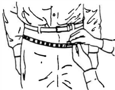
**Figure 5:** Position of belt and strap when climbing
