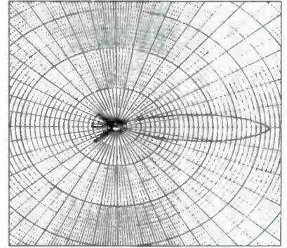
radiating elements, forming antenna arrays. Elements can be phased to give the various azimuth distributions and beam tilts below horizontal. Increasing gain is realized by stacking an increasing number of "bays" or shorter tubes.
