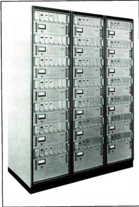
**Setup of transmitters for a 21-channel wireless cable system.**
