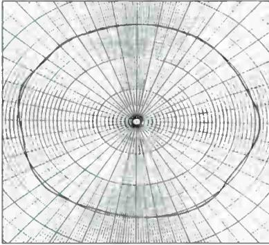
**Figure 4:** Horizontal plane radiation pattern for hemisphere coverage
