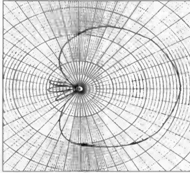
**Figure 5:** Vertical plane radiation pattern for hemisphere coverage
