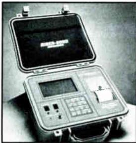
Cable Fault Locator
