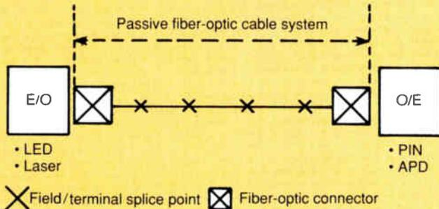
**Figure 2: Typical end termination detail (not to scale)**
