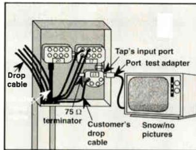
DC-30 and unacceptable signal levels or picture quality at the tap port indicate a defective DC.
