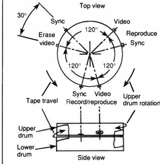
the drum diameter and speed, the tape width and the tape speed. Three of the tape wrap configurations are shown. The omega wrap and alpha wrap are full wrap types. A complete TV field is recorded with each revolution of the drum. With the half wrap configuration, a complete field is recorded with each half revolution of the drum and alternate fields must be recorded with different heads. Half wrap is universally used with cassette recorders because of the ease of threading.
