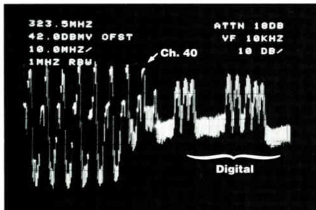
SkyPix channels can occupy in the cable system. Analog video channel assignments are placed in a data base to allow the controller software to determine optimal digital channel structuring (within available spectrum) for minimal intermodulation distortion of all carriers (both analog and digital video). This information also is required at the receiver to facilitate digital vs. analog tuning discrimination.
