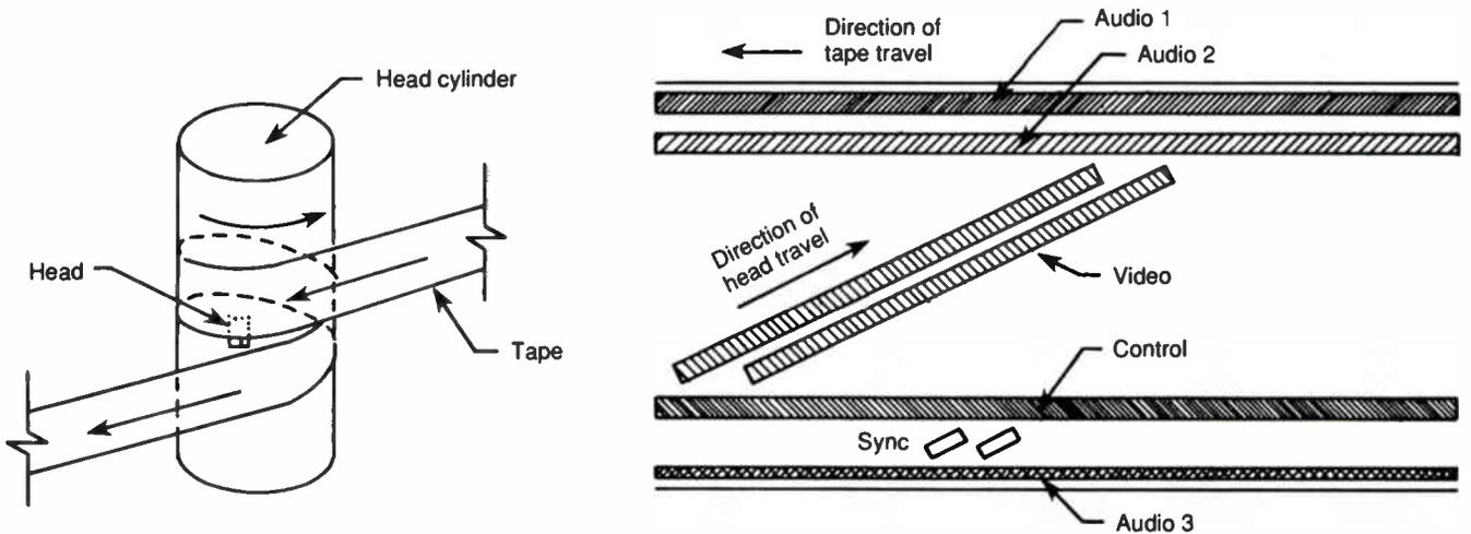
**Figure 3: Helical tape wrap configurations**
