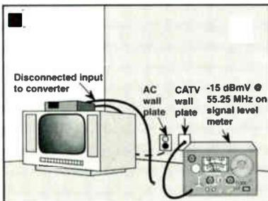
**Figure 3:** Checking at the wall plate with customer's TV set
