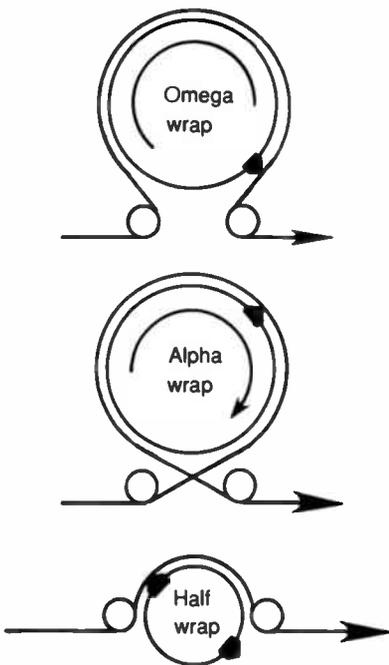
**Figure 4: SMPTE Type C head layout**
