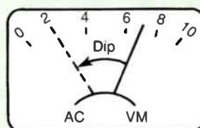
Shorted winding indicated by dip in AC voltage reading
