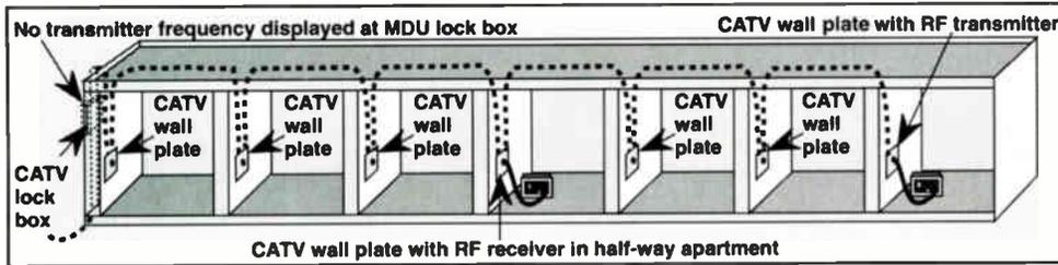
is halfway between the CATV lock box and the customer's apartment. Go to the halfway apartment to check for the presence of the Cable Designer RF transmitter frequency at the output cable of the directional coupler by removing the CATV wall plate, disconnecting the output cable from the directional coupler, and connecting the output cable to the Cable Designator RF receiver (Figure 17).
