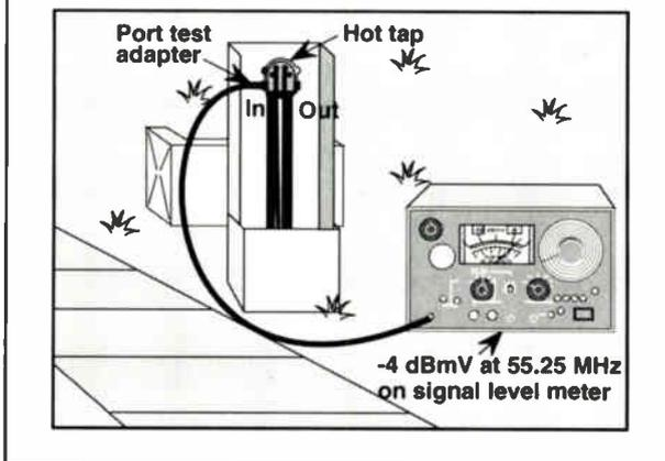
able video carrier signal level or poor picture quality at its output port indicates a defective DC.
