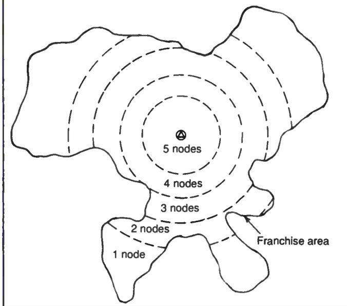
port further subdivision of the serving areas. The design is most cost-effective when the serving area is equal to or greater than 12 miles of plant.
