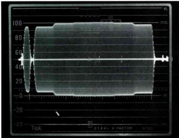
With the luminance portion of the signal filtered out, differential gain errors become obvious. This waveform has about a 10 percent differential gain error.
