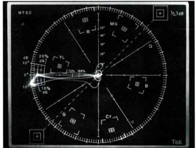
Some vector scope graticules feature special markings for measuring differential gain and differential phase. This signal has errors of approximately 10 percent differential gain and 9° differential phase.
