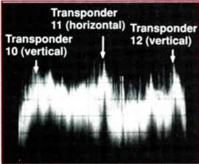
In this example we are looking at an LNA that is used to receive the satellite's vertically polarized signals, and will rotate the feedhorn to minimize the amplitude of horizontally polarized signals.
