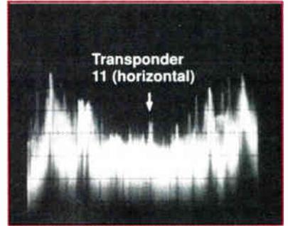
**Figure 7:** Lowest amplitude achievable with this particular earth station
