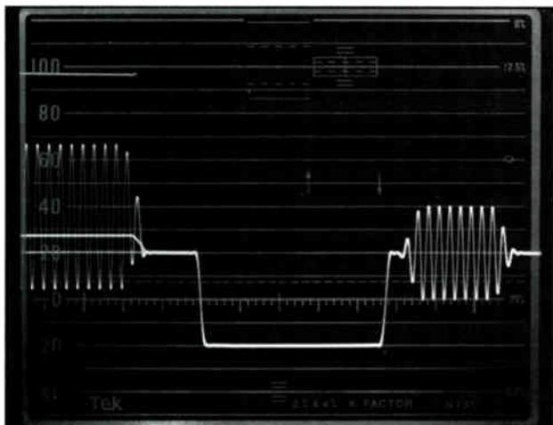
Sync timing requires establishing a reference position for the leading edge of sync on the reference signal.
