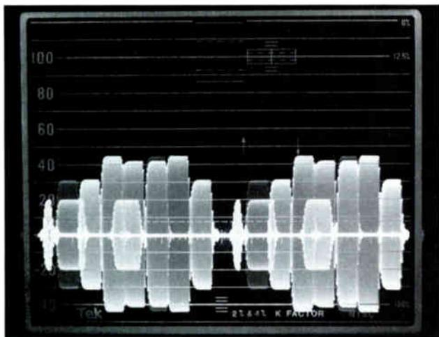
The chroma filter removes all luminance from the display. It is used for measuring chrominance levels and distortions.
