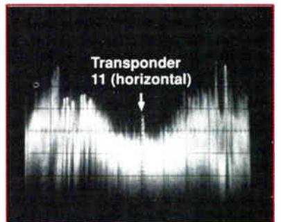
In this case, cross-polarization isolation is more than 20 dB.
