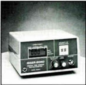
**Cable Fault Locator**
