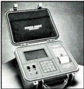
**Cable Fault Locator**
