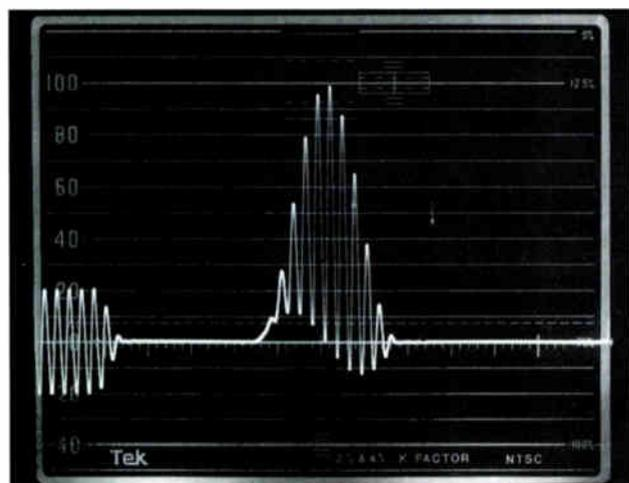
The sinusoidal distortion in this pulse's baseline indicates 250 ns chrominance delay.
