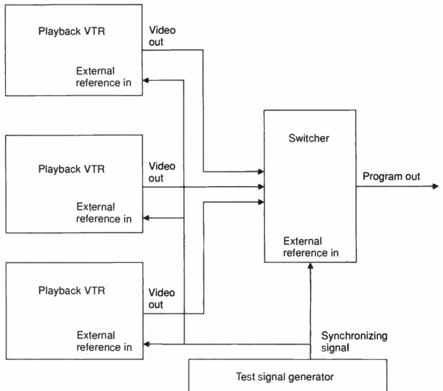
A simple synchronous system requires a common external reference for each component in the system.
