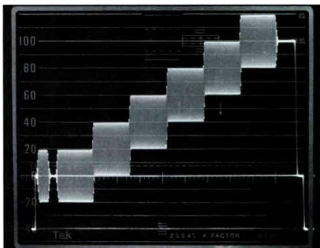
The modulated staircase signal is used for checking differential gain and differential phase.
