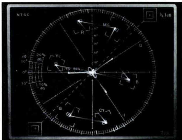
A properly adjusted vectorscope display will have the color burst in the nine o'clock position. Color bars signal amplitude is correct when all dots are in their boxes.
