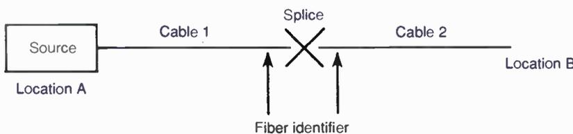
**Figure 3: Measuring end-to-end loss between connectors in a point-to-point fiber-to-the-curb installation**
