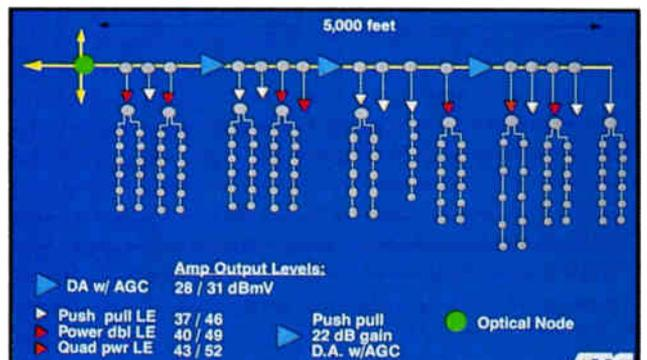
**Figure 5: Single cascade high output LE FTF architecture at 550 MHz**
