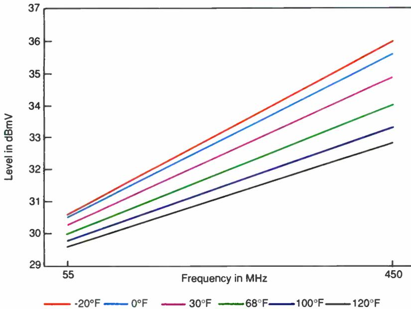
temperature is -20°F and the cable loss is 20 dB, which pad and equalizer should be selected? A 1 pad and 19 equalizer at 68°F would be the correct choice:
