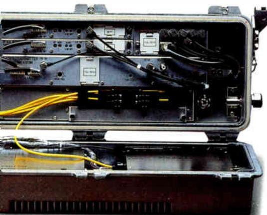
*Our new, economical VSB-AM strand mount optical receiver frees you to create fiber-to-feeder and fiber-to-line-extender architectures.*
