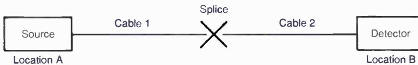
**Figure 2: Local detection of transmitted power for monitoring splice continuity**
