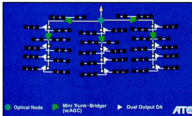
860 MHz architectures have evolved over the last 10 years. Figure 9 shows an architecture that was built in France approximately 10 years ago. This approach strongly resembles the super distribution architecture. While all of these European systems were designed for channel loadings of 20 to 50 channels, the architecture comparison is valid since the cable attenuations and passive losses at 860 MHz are very close to those at 1 GHz. Since the performance of the amplifier technology used
