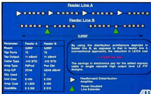
**Figure 8: Low-density build using optical supertrunk**
