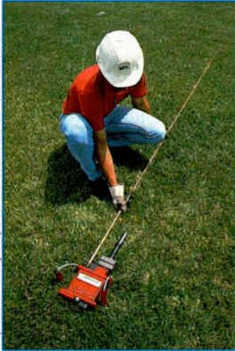
**Photo 1:** The ground rod is inserted into the Sidewinder's jaws.
