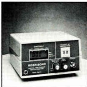
**Cable Fault Locator**
