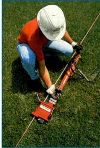
**Photo 2:** The jackhammer is placed on the Sidewinder's shank.
