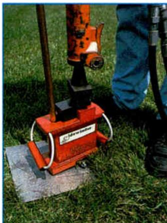
**Photo 6:** The Sidewinder's jaws are released from the rod.
