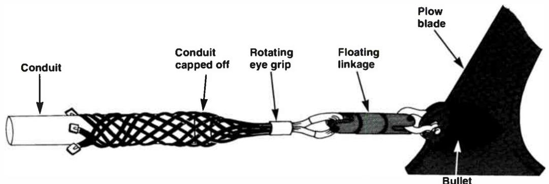
ground (Figure 6 on page 33) as the plow cuts through the ground between the pedestal sites. This last method works best unless obstacles are encountered that would require following the first method from that obstacle on to the next pedestal.
