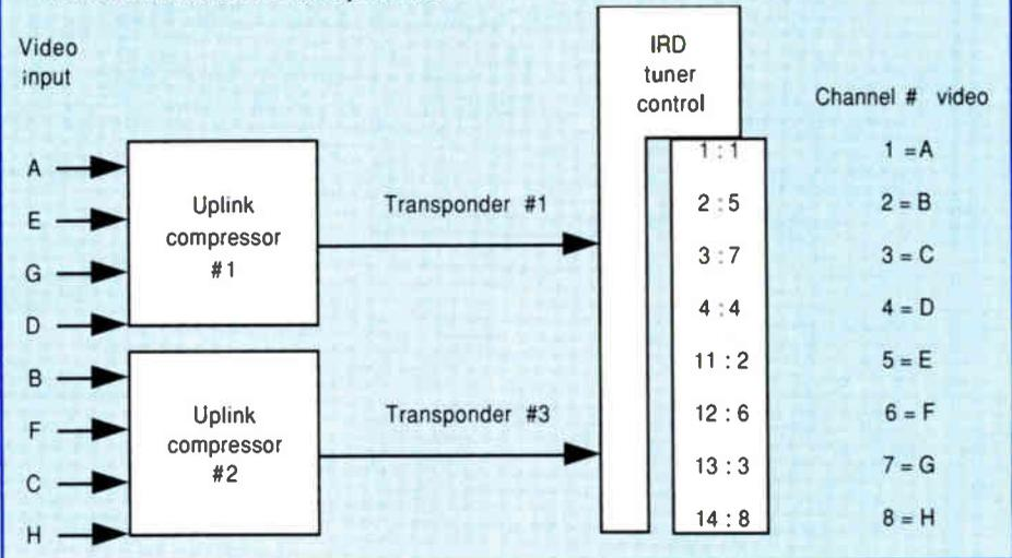
screen guides is a major step in turning the confusing array of video, audio text and data options into viewer satisfaction.
