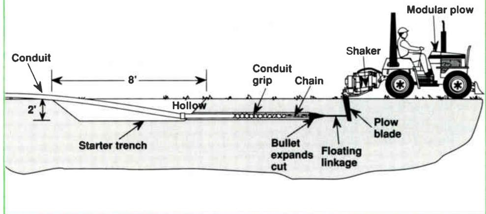
conduit to the plow blade with a pulling grip (Figure 7 on page 33); and 4) pull the conduit into the ground using the vibratory plow (Figure 8). Be sure to pull the coaxial cable into the conduit before backfilling the starter trench.
