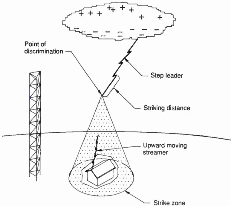
stroke. This accounts for the strange phenomena of a stroke hitting a small building at the base of a tall tower equipped with a lightning rod.
