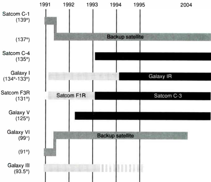
gramming to accommodate protected cable services in the event of fleet satellite failures.
