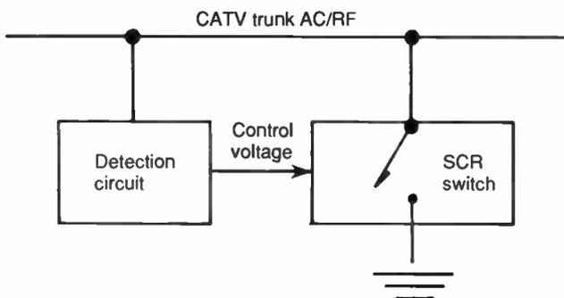
**Figure 2: 400 V spike caught at 104 V and grounded out in 0.5  $\mu$ sec**
