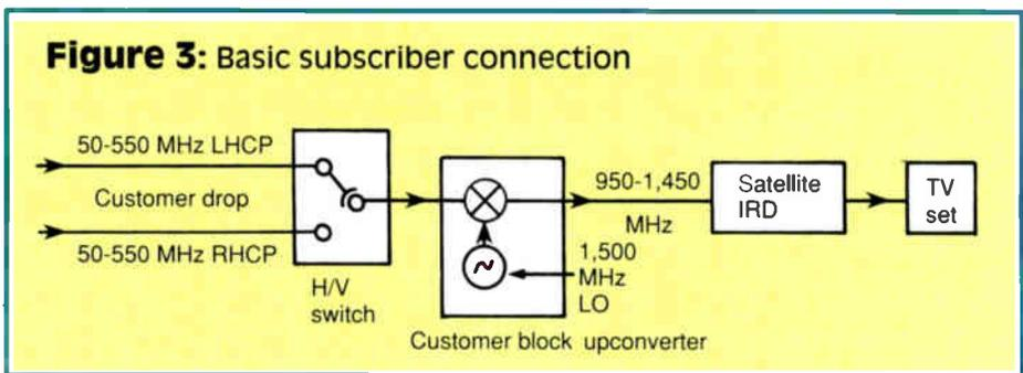
local programming in NTSC format could be either diplexed off the cable and fed directly to the TV set, or (more desirably) it could be transcoded into the digital satellite format at the headend and also be received through the IRD.
