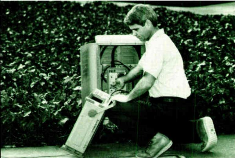
**HP's portable CATV analyzer speeds up troubleshooting.**
