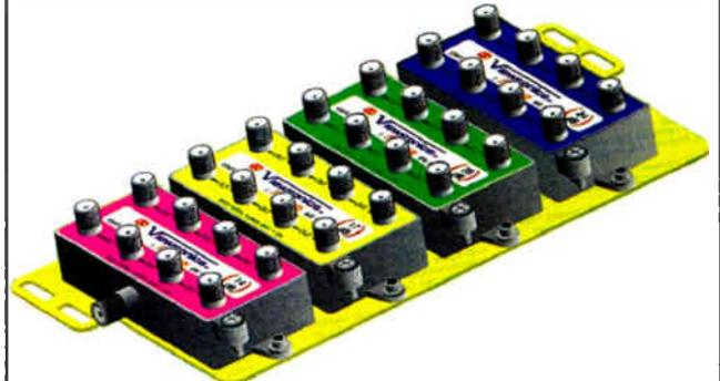
Viewsonics introduces a new concept in multi-output distribution taps. Using a modular concept, they developed a series of multitaps having various port values within the 16, 24, 32, and 48 port models. Home-run installs with extreme distance variations are easily served. In addition they provide for more selectivity in signal level. Tap values are from 14 to 35dB, from 5-600MHz.
