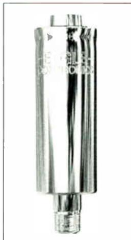
Jamming carrier positive traps inherently lose some video. This new trap has a narrower notch resulting in less video loss and sharper pictures. Immediate improvement for current systems can be realized while dramatically increasing the number of positively trapped channels.
