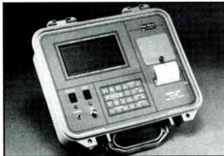
MTDR-Cable Fault Locator
