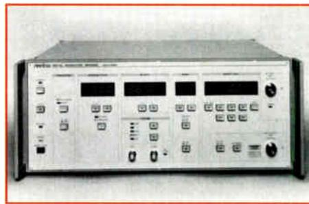
to 320 kb/s and can generate four types of patterns, including the PN9 and PN15 pseudo-random patterns required for modulation. The MN3650C's baseband signal sources can select 11 types of bit rate in a range of 32 kb/s to 384 kb/s.
