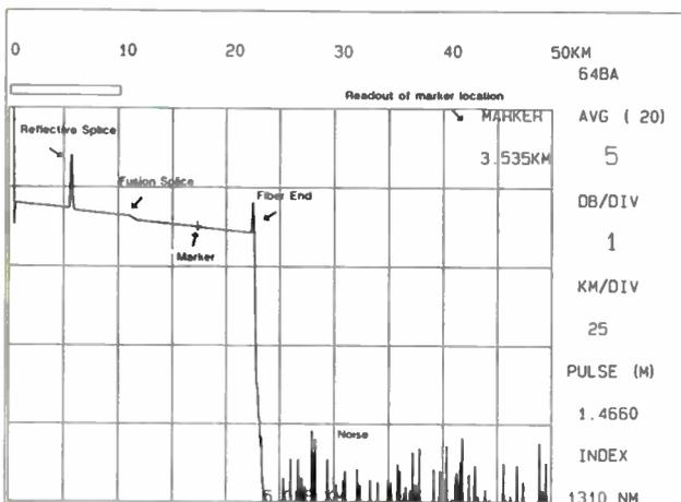
**Figure 3: A reflective fiber break**
