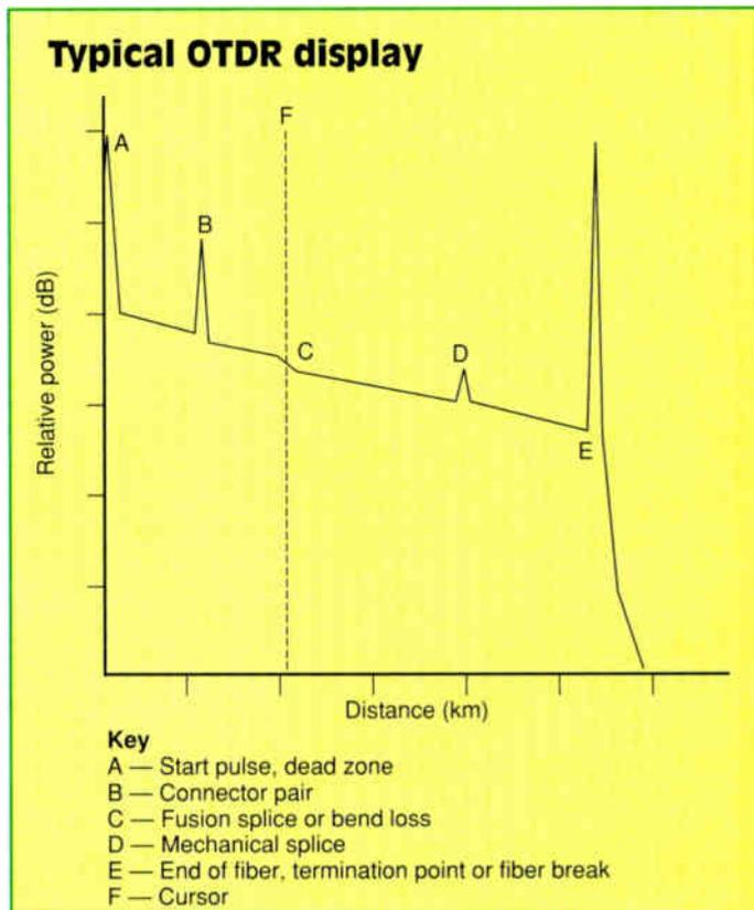
1,310 than at 1,550 nm, the fiber is much more bend-sensitive at the longer wavelength. It would be unfortunate to find that a system operating at 1,310 nm is obsolete at 1,550 nm, prohibiting future enhancements such as wavelength division multiplexing.
