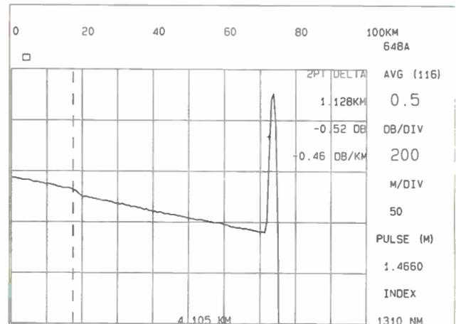
to 1,550 nm. On a long fiber you also should let the OTDR average for longer than a minute.
