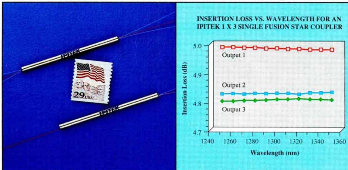
Now IPITEK offers *Single Fusion*  $N \times M$  single mode star couplers. Using our *Single Fusion* approach to  $N \times M$  configurations provides several advantages when compared with conventional tree couplers. Fewer splices increase system reliability. Excess loss is lowered. Best of all, the whole package fits in the same space as a standard  $1 \times 2$  coupler. Clean up your splice tray and improve system performance with quality *Single Fusion* star couplers from IPITEK.
