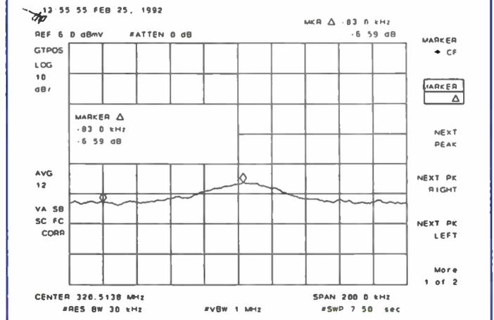
An analyzer measures in the units of dBmV for a large dynamic range. After doing some algebra one can calculate:
