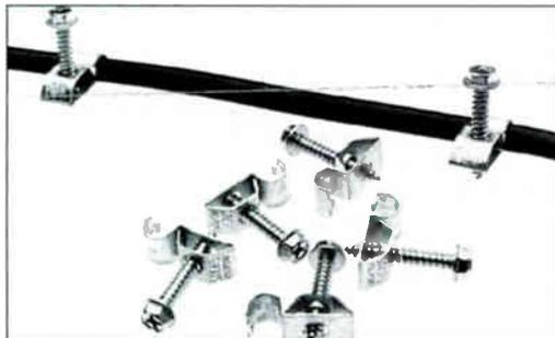
The SC 16 "SAXXIT"™ metal cable clip is made of weather resistant galvalume steel and is used for securing and maintaining a uniform installation of the coaxial cable onto most surfaces via its pre-inserted self-tapping screw or drive pin.
