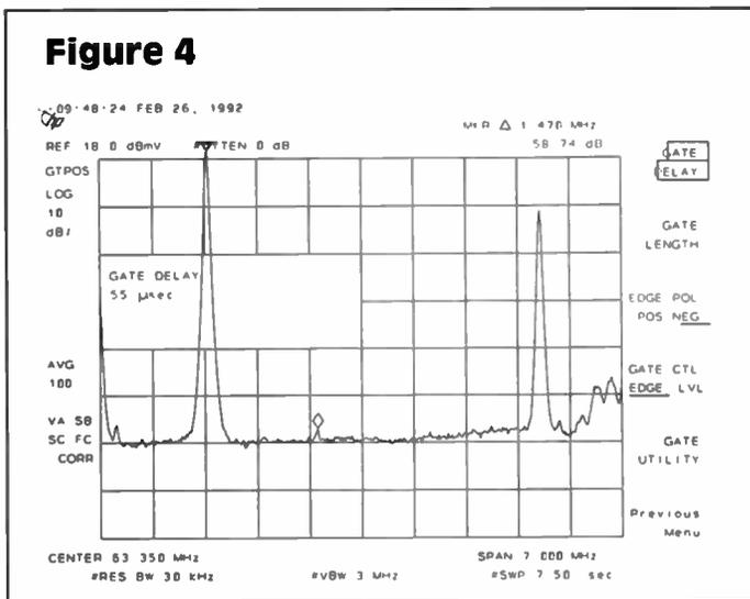
**“The ability to view a signal’s spectrum at a specific instant in time in the presence of modulation is key to the non-intrusive diagnosis of cable TV system problems.”**
