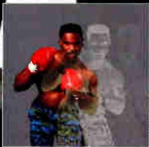
Test image with two multipath distortion echoes
