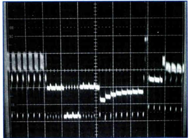
**Figure 16:** Shift of sync tips in vertical blanking
