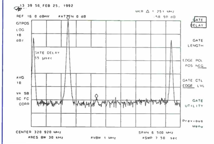
spectrum analyzer used for this article. We must make sure that we get at least one burst per bucket. If this is not the case there will be dropouts, or zero values, in some of the trace elements. Video averaging improves the accuracy of the noise floor measurement at the expense of measurement acquisition time.
