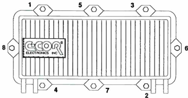
2) Close the cover until it is flush with the rubber gasket. Refer to Figures 1 and 2 for the tightening sequence for four- and eight-port housings. Thread all cover bolts finger tight to hold the cover in place. Ensure that it seats evenly on the rubber gasket.
