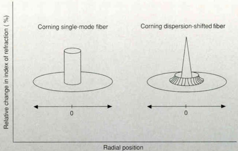
the fiber core. (See Figure 3.) The refractive index profile represents the change in refractive index of the core glass relative to the cladding glass, and typically defines the fiber's transmission characteristics.
