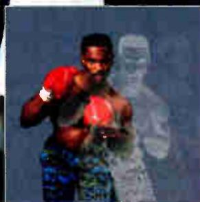
Test image with two multipath distortion echoes
