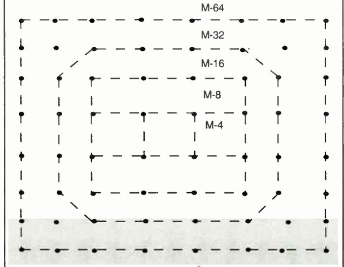
ture amplitude modulation (QAM). QAM signal waveforms are a form of combined amplitude and phase modulation. Several different constellation diagrams for QAM are illustrated in Figure 7 for  $M = 4, 8, 16, 32$  and  $64$ . We observe that the QAM signal waveforms result in rectangular signal space constellations when the amplitude values on the two quadrature carriers are equal.
