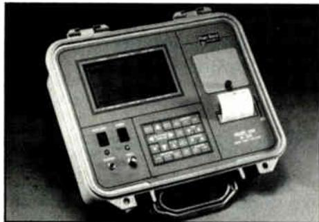
MTDR-Cable Fault Locator
