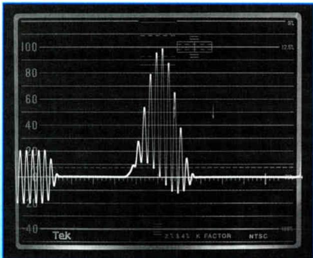
A sinusoidal distortion in the base of the 12.5T mod pulse indicates chrominance-to-luminance delay. In this example chrominance is delayed by approximately 250 ns.
