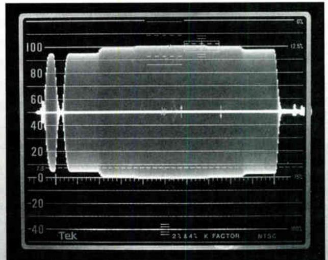
This modulated staircase signal exhibits a 10 percent differential gain error.
