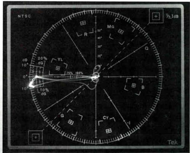
This vectorscope display shows simultaneous differential gain and differential phase errors of 10 percent and 9°, respectively.
