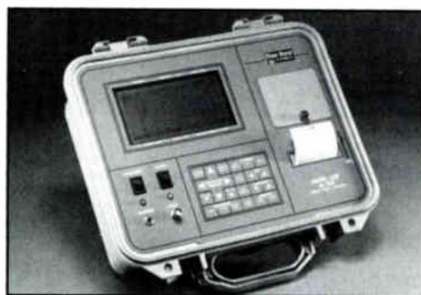
MTDR-Cable Fault Locator
