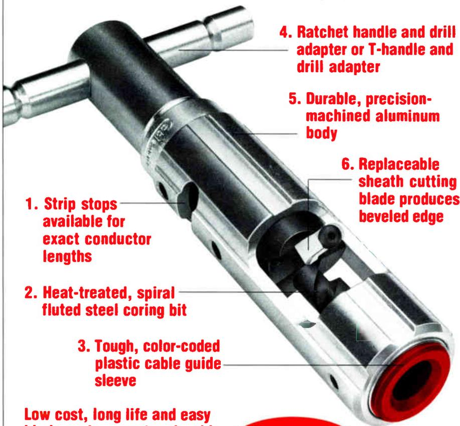
1. Strip stops available for exact conductor lengths
