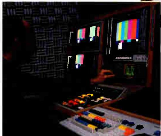
(RIGHT) A WAVEFORM MONITOR, VECTORSCOPE AND NTSC GENERATOR CONSTITUTE A LOW-COST SYSTEM FOR EFFECTIVE BASEBAND MONITORING.
