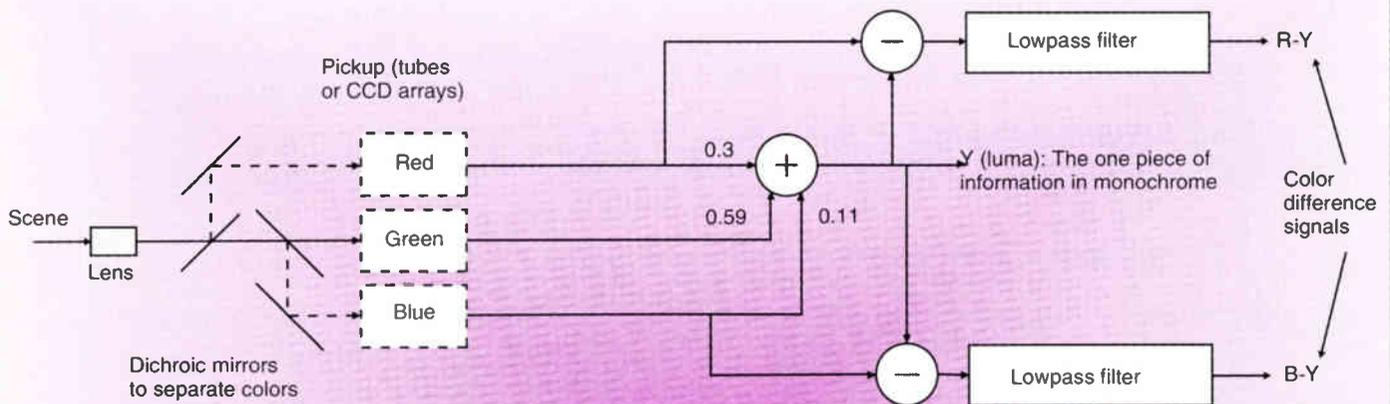
**A: Generation of analog components. This is the starting point for both NTSC and digital compressed video.**
