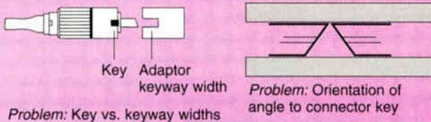
carefully the connectors are taken apart and remated. APC connectors, on the other hand, reflect light back at an angle. Angles anywhere between 6° and 12° seems to be optimum. This reflected light then exits the fiber. Any minor scratching has no effect on backreflection. See Figure 3 and Table 2 on page 46.
