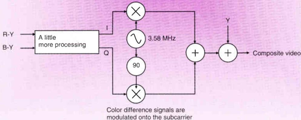
**B: Processing of the video into the NTSC format**
