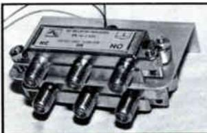
This is a picture of our DPDT RF relay. It switches frequencies from DC-600 MHz with ease. We use it to build RF switching systems ... SPDT, DPDT, 4PST, 4PDT and so on. No nonsense. It has very high isolation and very low insertion loss. These units are now switching signals in some very large cable TV headends for testing and/or routing purposes. Our relays can help you do your job better, too. No nonsense. Call or fax for free info. on all our products.
