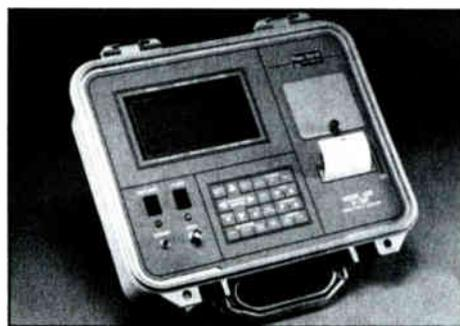
MTDR-Cable Fault Locator
