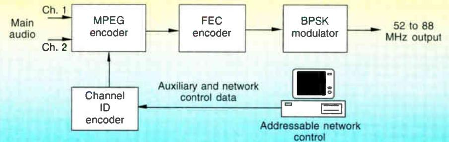
**Figure 2:** Typical MPEG digital audio single channel per carrier receive block diagram
