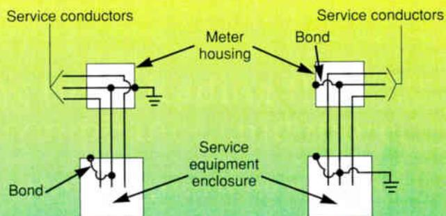
On the left is a grounding electrode conductor at the meter housing with the service equipment enclosure bonded to the grounded service conductor. On the right is the grounding electrode conductor at the service equipment with the service equipment enclosure and the meter housing bonded to the grounded service conductor.
