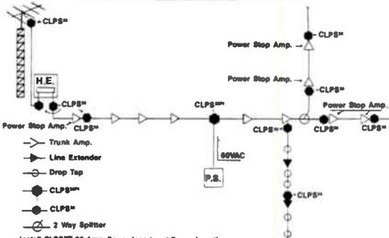
Install CLPS<sup>35PI</sup> 35 Amp. Power Inserter at Power Insertion.
