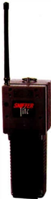
hum and carrier-to-noise. You can examine your system at any level of detail you require. All channels will be viewable with your choice of models—5 to 860 MHz or 50 to 860 MHz.
