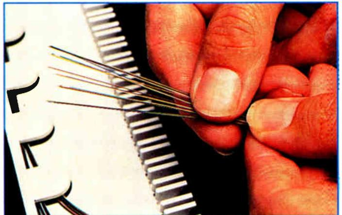
Although it's impossible to work with fiber and not bend it, steps should be taken to follow manufacturer's guidelines on bending.
