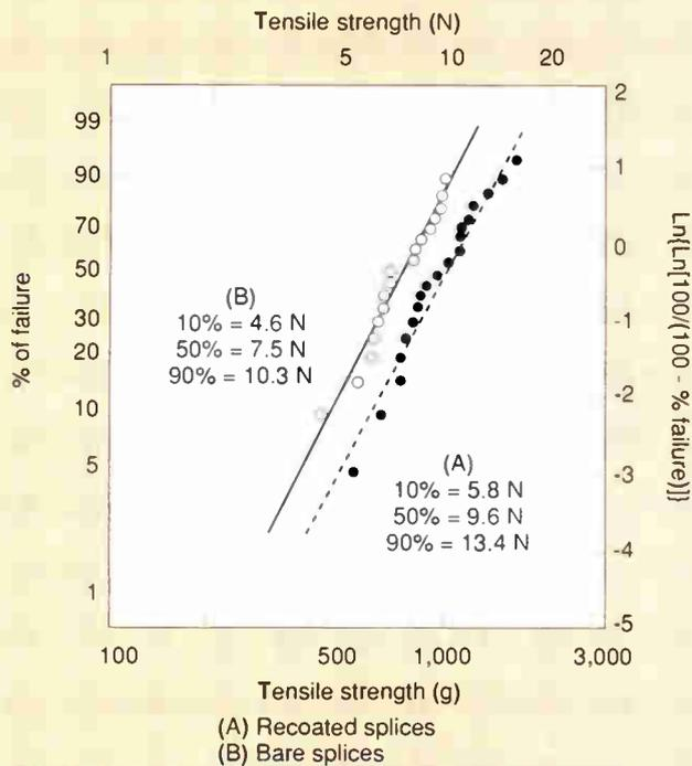
**Figure 5:** Effect of aging on tensile strength of single-fiber recoated fusion splices
