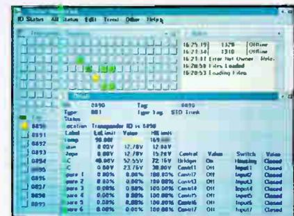
Network Manager controller transponder alarm detail screen.
