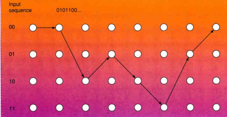
tions for the rate 1/2 coder of Figure 5a. From an inspection of Figure 6, it is seen that transitions between certain states are not possible. For example, a transition from state 00 to state 11 cannot occur because shifting a 1 into state 00 causes the contents of the first shift register location to be 0 and not 1.
