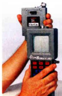
Wavelength selection is made by choosing a softkey on the face panel of WindowLite PLUS.
