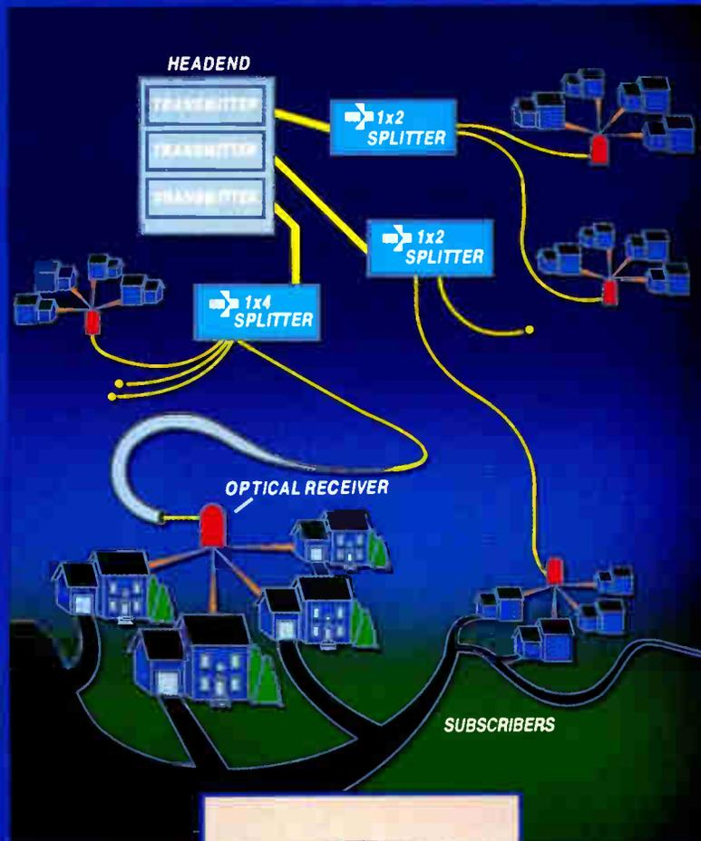
For CATV systems Gould has wavelength independent splitters with low insertion loss and high directivity ( $\leq -65.0\text{dB}$ ) -- guaranteed for environmental stability and performance at the headend or in the field. Components are in stock in a variety of standard and customized package styles.
