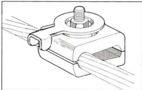
**Universal support for any bail type drop wire clamp or 3-6-3 wrap... and mechanically galvanized!**
