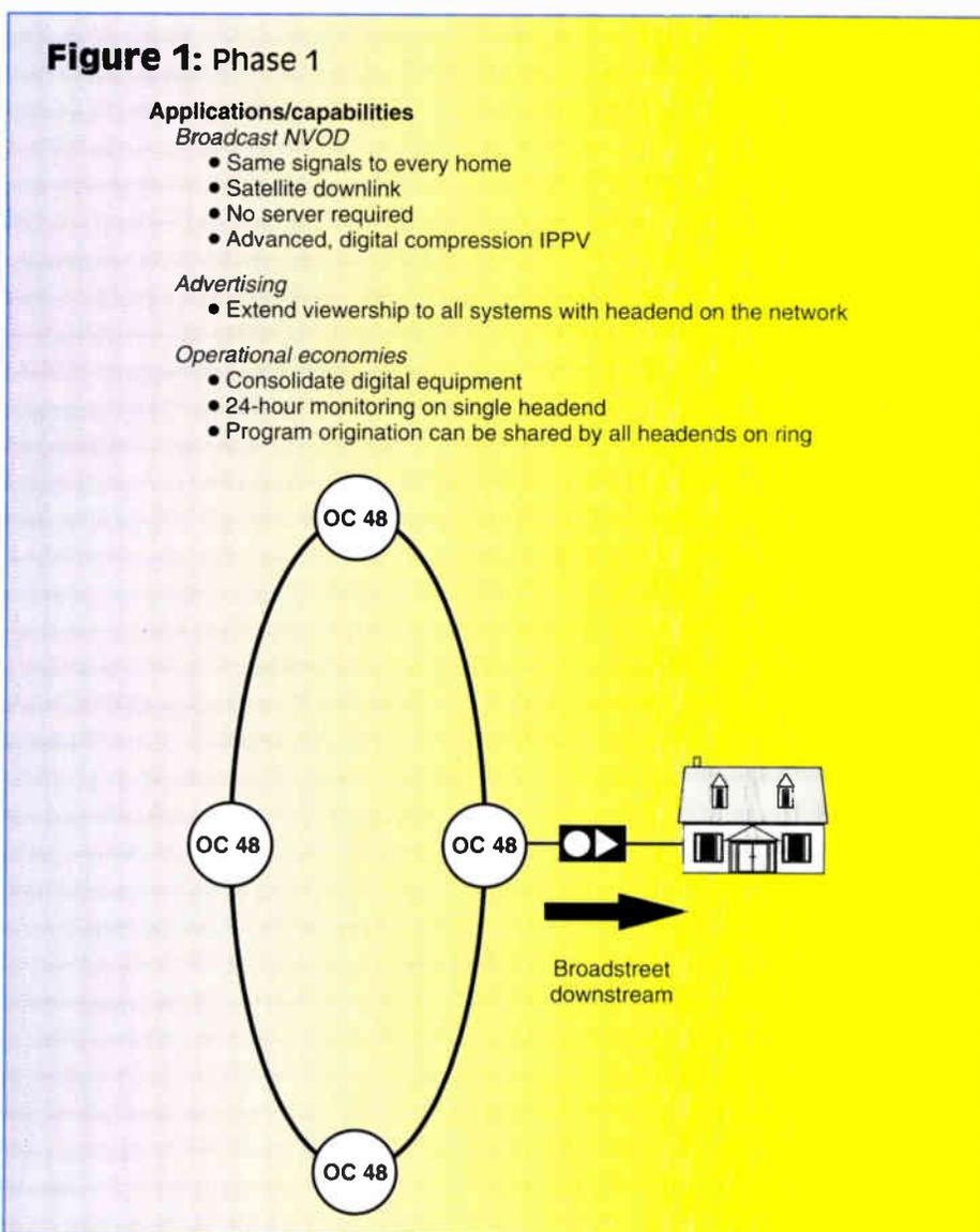
nect existing cable TV headends and gain seamless access to the public switched telephone network (PSTN). SONET is, in essence, a digital "super-highway," able to seamlessly pick up and drop off traffic at any node in the network. SONET's self-healing ring architectures are capable of protecting the traffic from a fiber break, equipment failure or catastrophic hub failure without any impact to telecommunication services.
