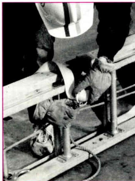
**3) Loop one end of the Ladder Tote around the ladder rail and the third rung from the center position.**
