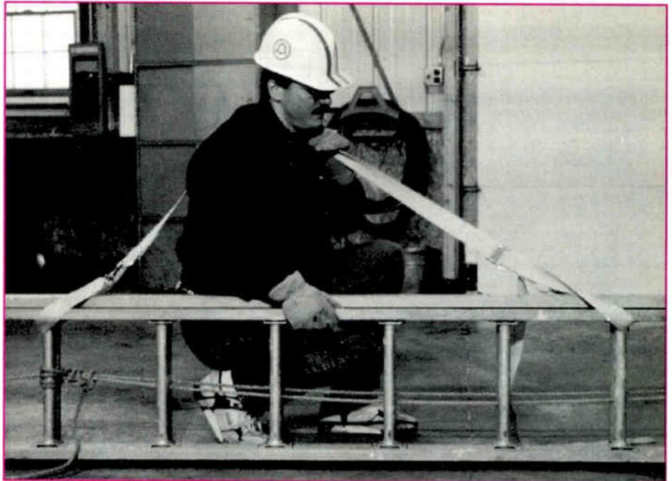
**7) Now the tech adjusts the Ladder Tote buckle removing slack until the ladder can be lifted and carried about hip-high.**
