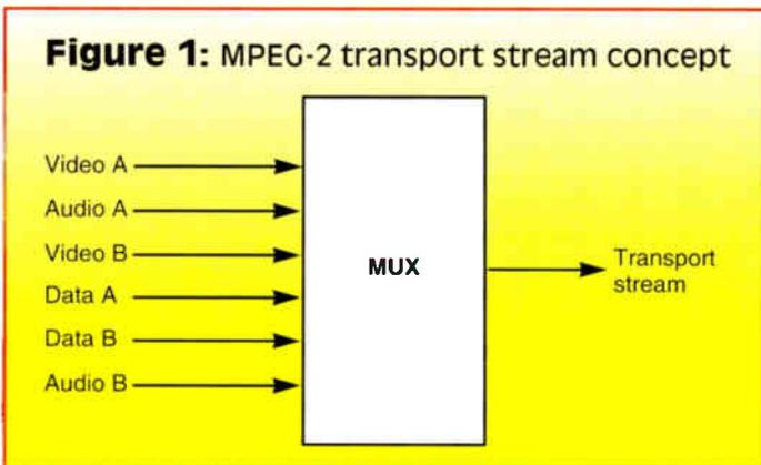
A prototypical view of the basic multiplexing concept of an MPEG transport stream is shown in Figure 1.
