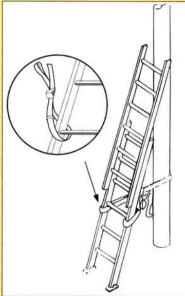
fore climbing and is the most commonly used because it is the quickest and easiest to use. The ITC-6003 has two quick release buckles for rapid setup and take-down. The ITC-6004 (Figure 2) does the same operation as the ITC-6003 except it uses straps around the ladder rail rather than hooks. Key benefits of using the Safe-Tie are:
