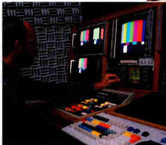
(ABOVE) THE 2714 CABLE TV SPECTRUM ANALYZER AUTOMATES ALL COMMON CABLE SYSTEM SPECTRAL MEASUREMENTS, INCLUDING THE FCC RF PROOF-OF-PERFORMANCE REQUIREMENTS.
