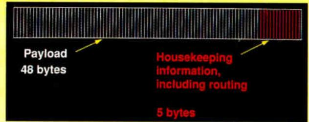
**Figure 5: Fast packet or cell switching**
