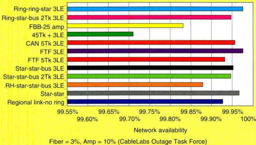
**Figure 4:** Availability of alternative network/plant configurations
