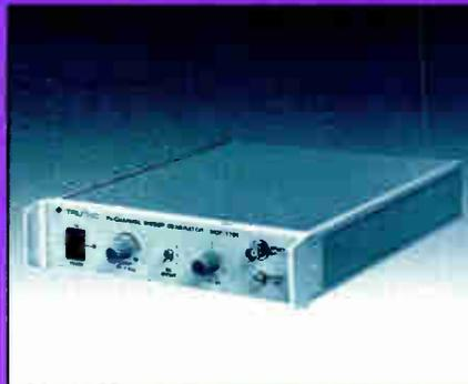
**NCC-1701** Video sweep generator, providing test signal to modulator for in-channel flatness of entire system. Use with any modulator and Trilithic SP-1075 or other spectrum analyzer equipped with digital storage
