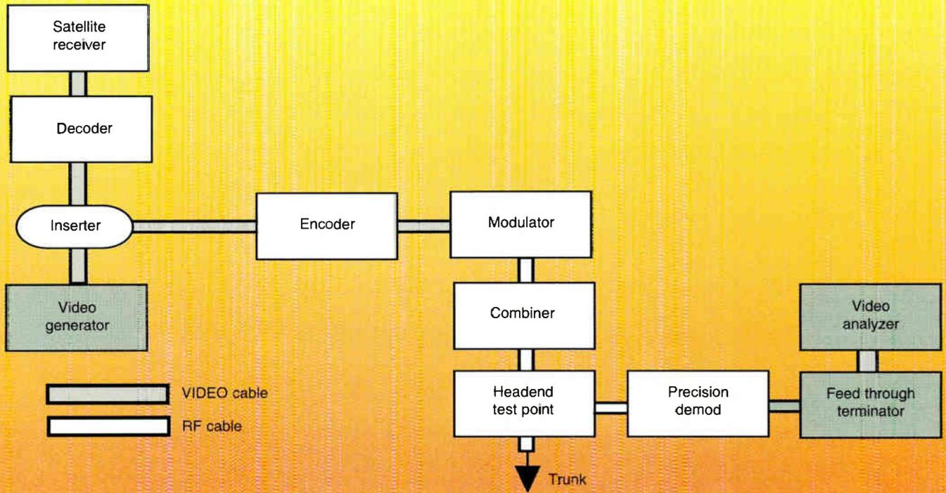
The maximum RF envelope amplitude occurs at the sync tips. The minimum RF envelope occurs at the whitest part of the picture. To properly measure or set the percent mod, the modulated carrier must contain both sync tip peaks and a 100 IRE white signal. If suppressed or stripped sync is used in your scrambling system, the scrambling must be turned off or a procedure permitting measurement of the unsuppressed sync during VBI must be used.
