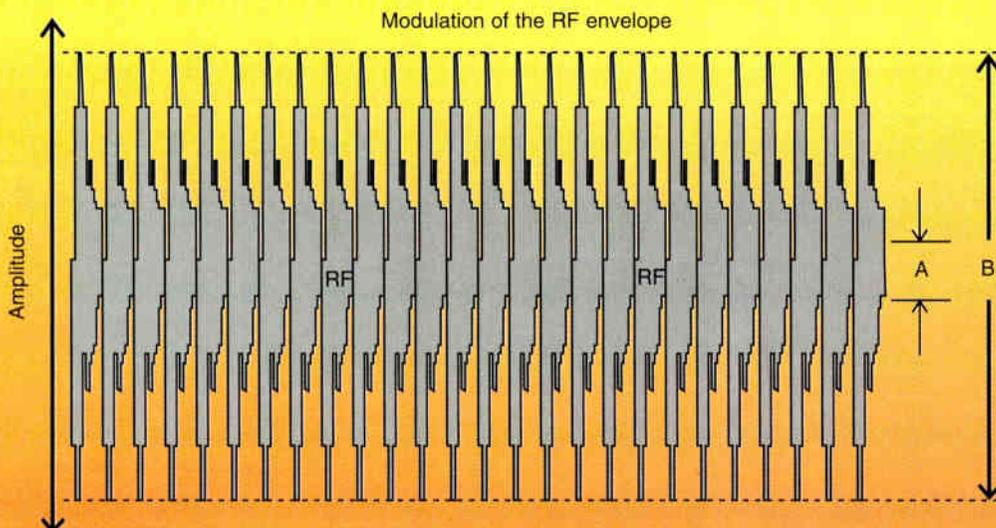
**Figure 13: Percent modulation measurement**
