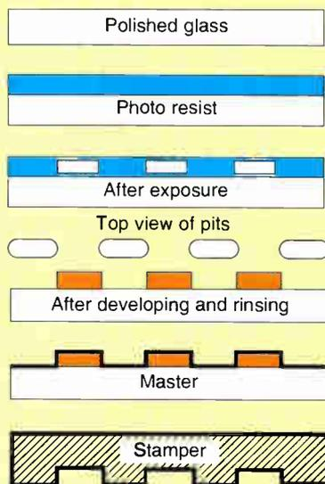
**Figure 2:** Mass production process for replicated laser discs
