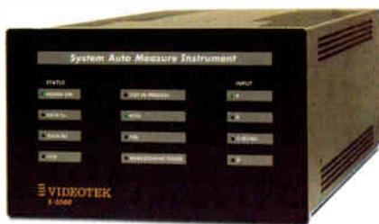
**S-2000 System Auto Measure.** The most affordable auto-measure instrument in the industry is also one of the most advanced. The S-2000 is capable of performing hundreds of NTSC and PAL video measurements with absolute accuracy.
