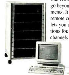
The NBT 9101 has features that go beyond the standard requirements. It comes with an extensive remote control PC program that lets you operate all of its functions for a single channel, all channels or groups of channels, fine tune the frequency of a channel, set a sloped output level, and recall instrument setups, and much more.
