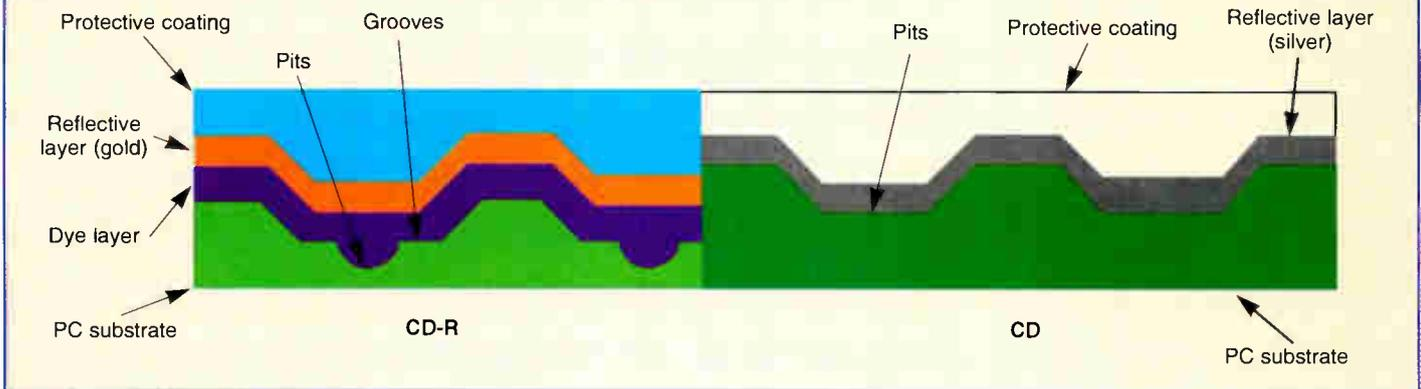
and track width of a CD are almost identical to those of the laser disc. The CD pits have a constant width of 0.5 micron, a depth of 0.1 micron and consist of nine different lengths ranging from 0.86 to 3.18 microns — the track width is 1.6 microns. The recording and playback of a CD is CLV and the track velocity is nominally 1.3 m/sec. A functional diagram of a read-only CD player is shown in Figure 4 (page 22).
