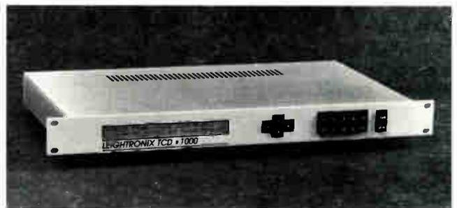
**Unattended program playback, recording and switching for local origination cable channels**
