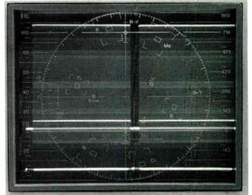
distortions are lower than the hum level you are attempting to measure. Hum distortion will commonly be a sinusoidal distortion at some low frequency (i.e., field or 2X field rate).
