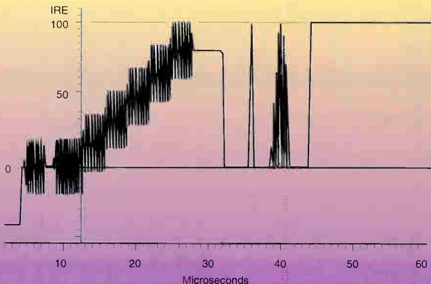
**Figure 6: NTC-7 composite signal**
