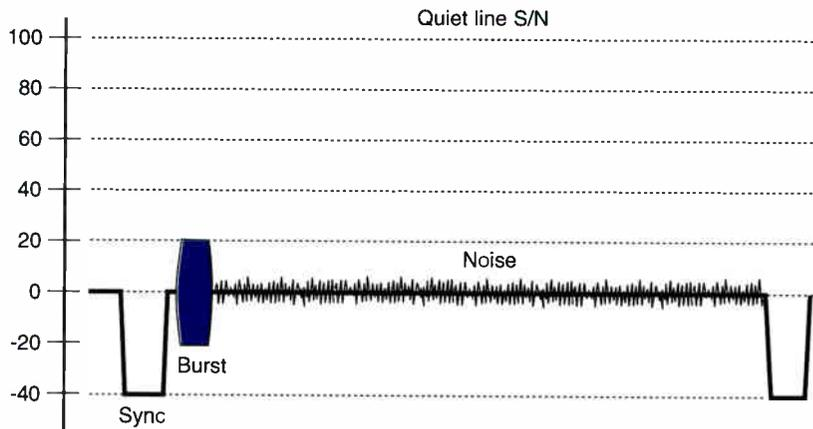
usually the result of poor video source material, an equipment failure, or when very distant off-air signals are brought in via marginal means. While most system sources of noise are flat across the spectrum, noise generated by imaging devices, microwave transmitters and satellite transponders is not flat. Generally, noise increases as the square of the frequency. This is a good reason to insert your own test signals using a VITS insertion generator.
