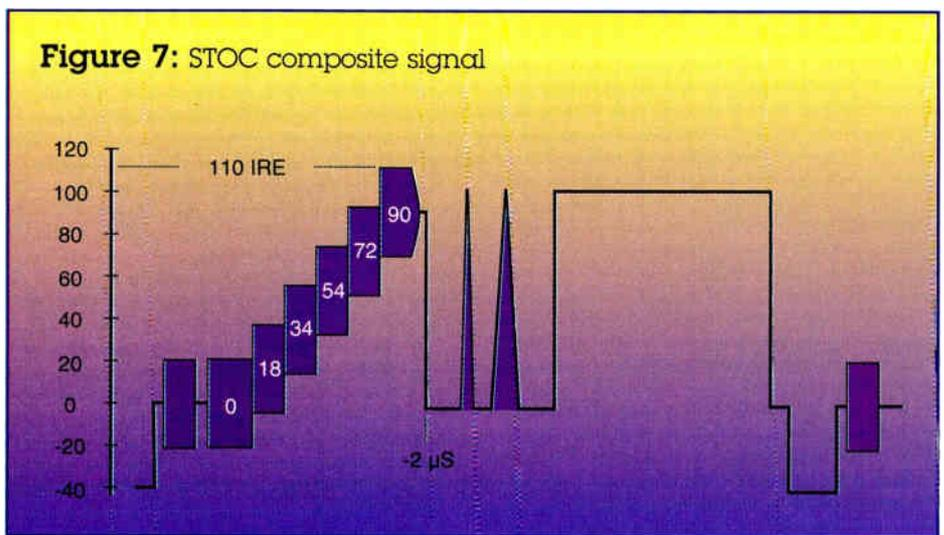
signal and can be easily mistaken for it. The differences, however, between the STOC and FCC composite signals are the chroma peak amplitude in the fifth stairstep, and a 2  $\mu\text{s}$  shift forward in time of the rest of the signal components after the fifth stairstep.
