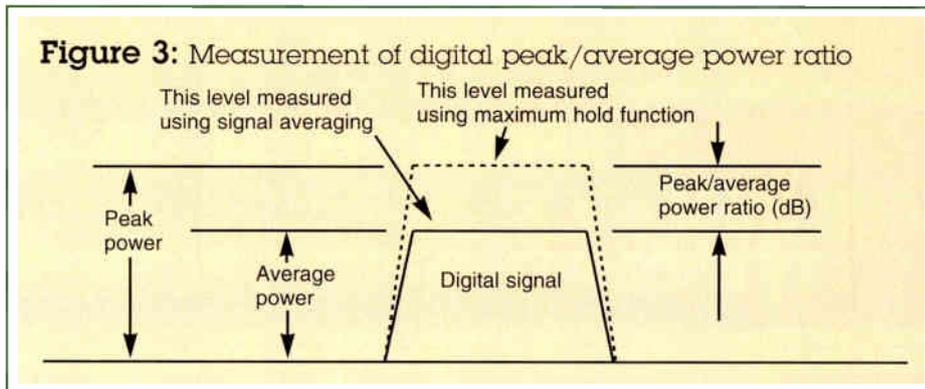
This measurement can be made rather easily if the analyzer incorporates both signal averaging and "max hold" functions. A number of analyzers have these features built into the instrument. If the analyzer is equipped with these, peak-to-average power ratios can be measured using the following procedure:
