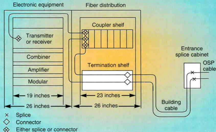
loss performance of splicing was preferred to optical connectors for attaching OSP cables to inside equipment. Early connectors also generated reflectances with magnitudes that caused discomfort because of the widespread uncertainty about their effects on AM systems. The prudent course was to minimize both loss and reflectance by using splices.
