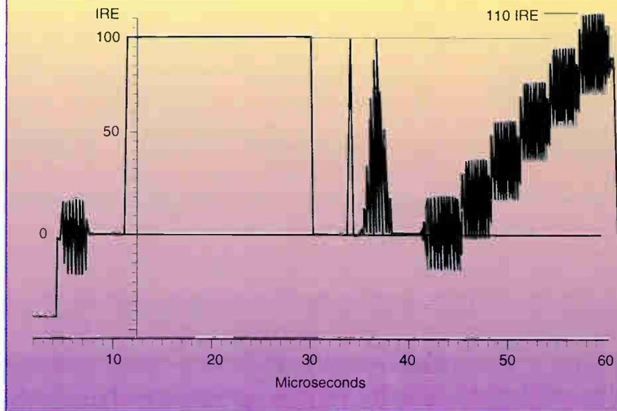
delay than the luminance signal so the test is probably named for this. However, negative delay, where the chroma component arrives first is not uncommon.
