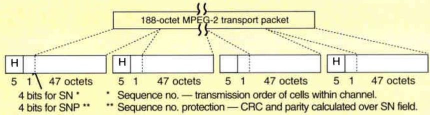
**Figure 6: AAL 5 adaptation of one MPEG transport packet**
