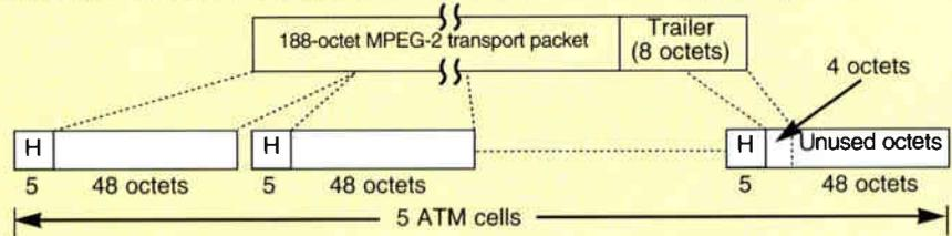
**Figure 7: AAL 5 adaptation of two MPEG-2 transport packets**
