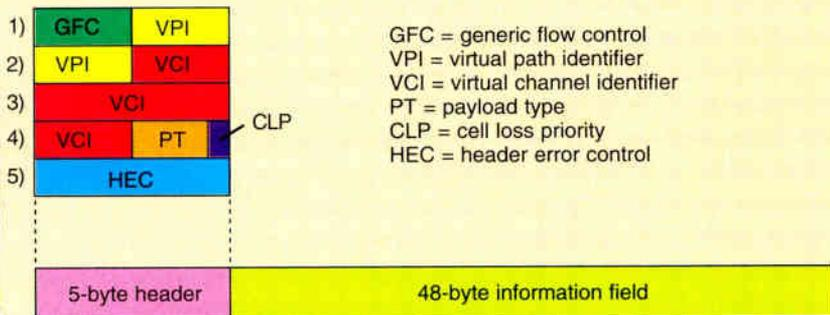
**Figure 4: Functions of ATM layers**
