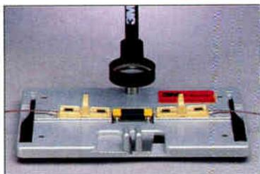
Fibrlok Multi-Fiber Splicing Assembly Tool
