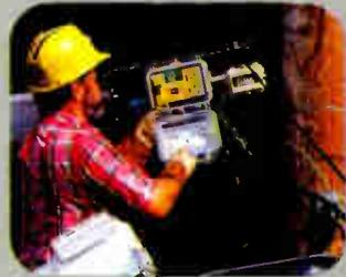
CALAN'S STAR 2010 Signal Level Measurement System heralds a whole new era in carrier analysis for the cable industry. A fast, accurate and easy-to-use instrument, The 2010 covers the entire frequency range (5 MHz to 1 GHz) with unmatched speed-36 channels in less than one second.
