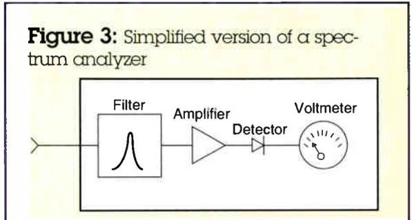
**Figure 3:** Simplified version of a spectrum analyzer
