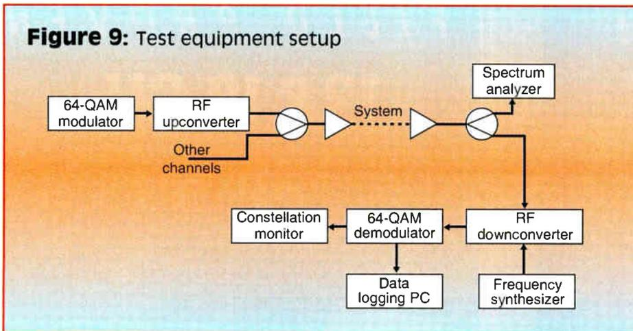
24-trunk amp cascade, plus two taps, plus considerable wiring to the receiving site (a hotel room). This test data includes a loss of signal due to an intermittent problem in the downconverter's power supply. See Table 2.
