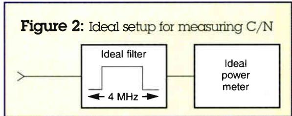
**Figure 2:** Ideal setup for measuring C/N
