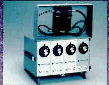
**VF-Series Filters/AM-600 Preamplifier** VF preselectors extend the range of composite triple beat, cross-modulation and carrier-to-noise measurements by filtering out all but the carrier to be measured. **AM-600** 20 dB preamplifier boosts set top converter output to level needed for FCC Part 76 testing.
