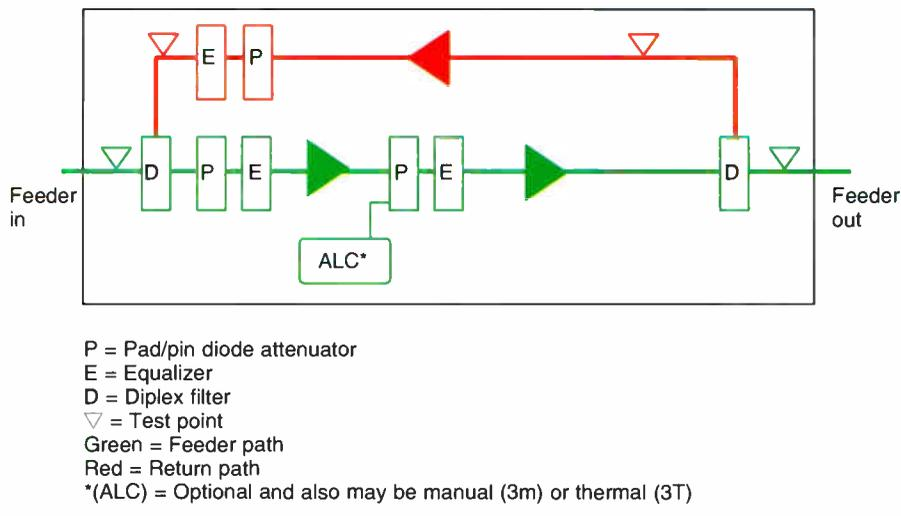
enough range to allow a technician to mask a system problem, albeit inadvertently, by permitting an amplifier to be set to the desired output levels in spite of an inadequate input level. All things considered, the pad and equalizer approach just seems to make a lot of sense to us.
