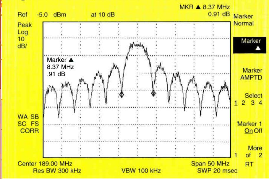
**Figure 3: Spectral sidebars removed**
