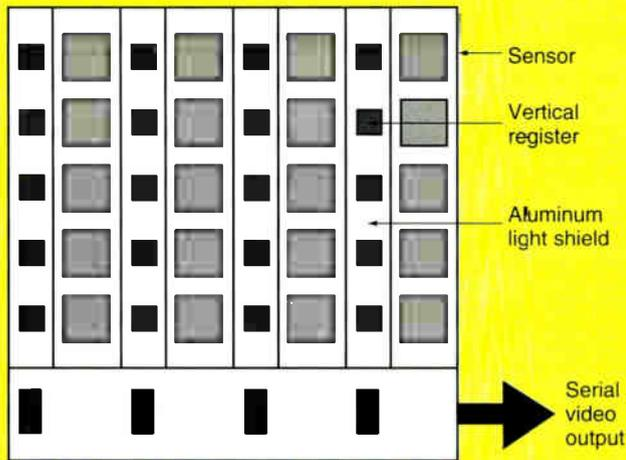
are used for photosensors and storage elements. See Figure 8. The shift registers are covered with an optically opaque aluminum mask. During field blanking all the charges generated in the photosensors are shifted sideways into the corresponding storage element. The storage array is then clocked out during the next field.
