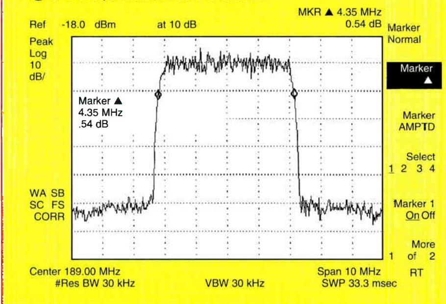
Ensuring the quality of service requires testing digitally modulated signals. As in an analog cable TV system, power and interference measurements are essential to maintaining digital cable TV services. Although the effects are different from impairments on an analog TV signal, amplifier compression and spurious interference will degrade digital video signals.
