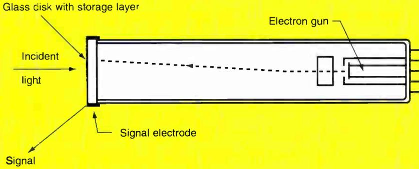
emitted. These are collected by the mesh. This leaves the glass membrane positively charged, and electrons are absorbed by the scanning beam. The return beam provides a negative image — that is, its current is highest in dark areas of the picture where very few electrons are absorbed from the scanning beam. The diameter of the image orthicon was 4-1/2 inches permitting use of standard lenses used in 35mm film cameras.
