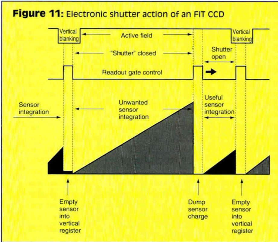
the electronic shutter action of the FIT CCD.
