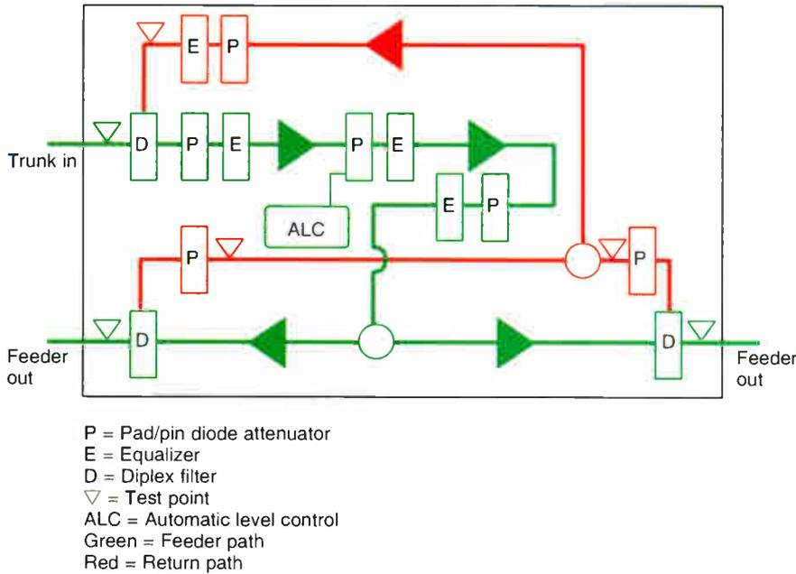
levels apply to the Type 2 amplifier, which can be used as either a terminating bridger or an intermediate bridger with an external splitter or coupler used to provide input signals. Line extender output levels are usually set to levels similar to those for the feeder ports of the Type 1 and Type 2 amplifiers.
