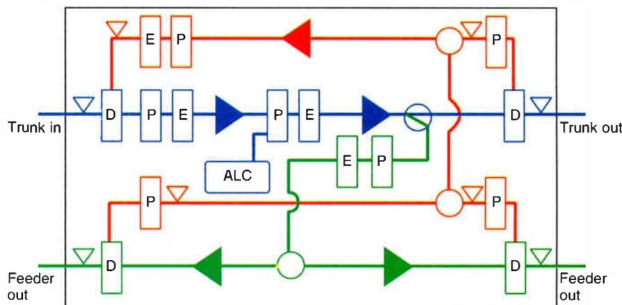
P = Pad/pin diode attenuator
