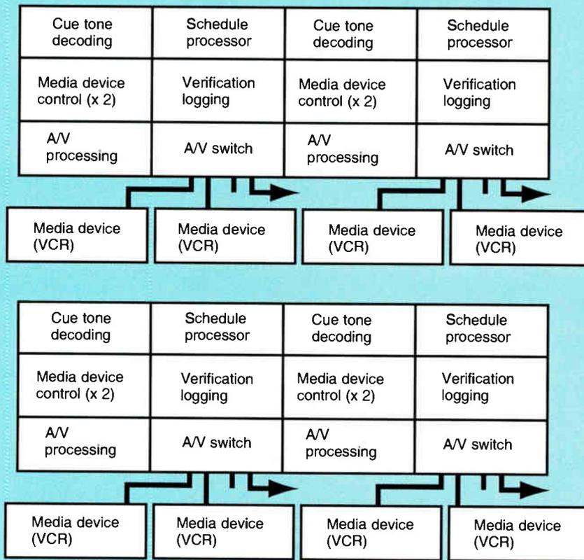
nels of insertion in a single self-contained rack-mount chassis. Each unit contained all the elements required for ad insertion. The circuits of the individual modules were consolidated on several larger boards, which reduced cost and increased reliability.
