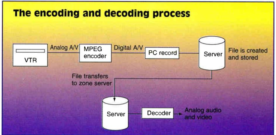
ty over conventional tape-based analog systems. The core technology involved in digital ad insertion is the set of digital video and audio compression techniques adopted as part of the worldwide standard called MPEG.
