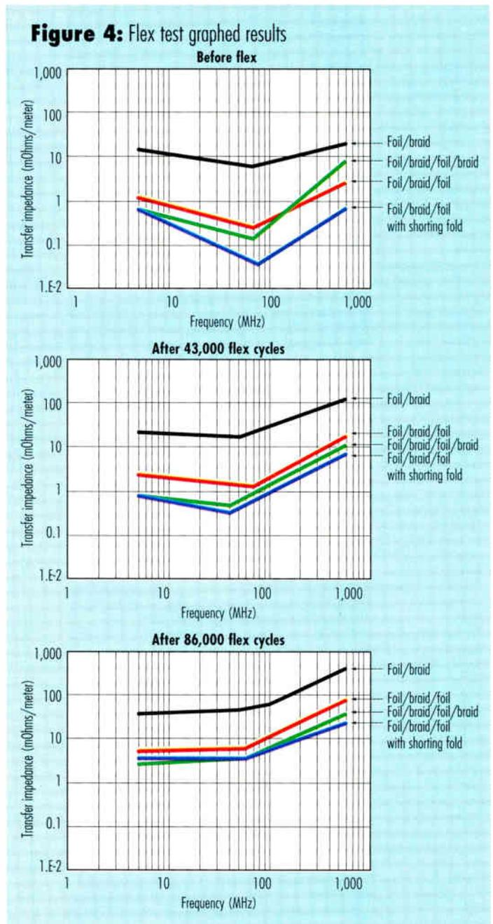
pendent upon the sample cable's shield construction. The lower the transfer impedance value, the more effective the shielding. Theoretically, the absolute interference level of a cable can be determined using the transfer impedance value. The transfer impedance takes into effect the relationship between the two signal-carrying regions of a coax cable. The shield separates these two regions. Therefore, the transfer impedance test is a true measure of the shield effectiveness of the cable.
