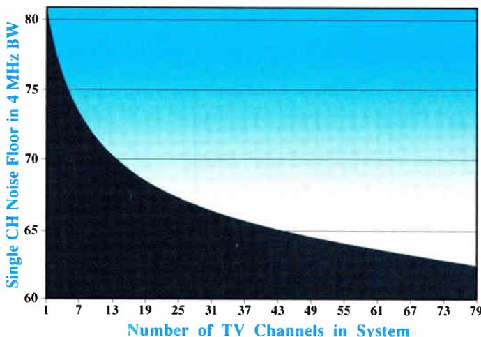
the gun and began marketing tuner synthesizers designed primarily for VCRs or set-top converters. These tuners provided agility, but at a significant cost in broadband noise. Also, because they were being pushed far beyond their design limitations, many other spurious signals came out in the modulator's final output. In the end, the industry labeled agile modulators, "for standby use only."
