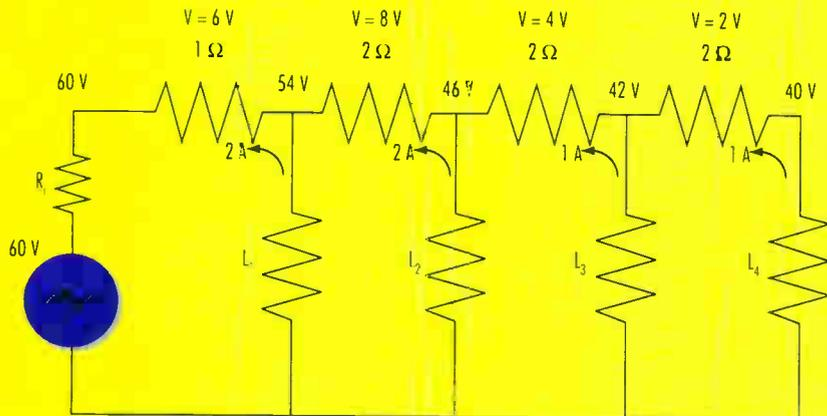
$$V_{R4} = I_{L4} \times R_4 = 1 \times 2 = 2 \text{ V}$$
