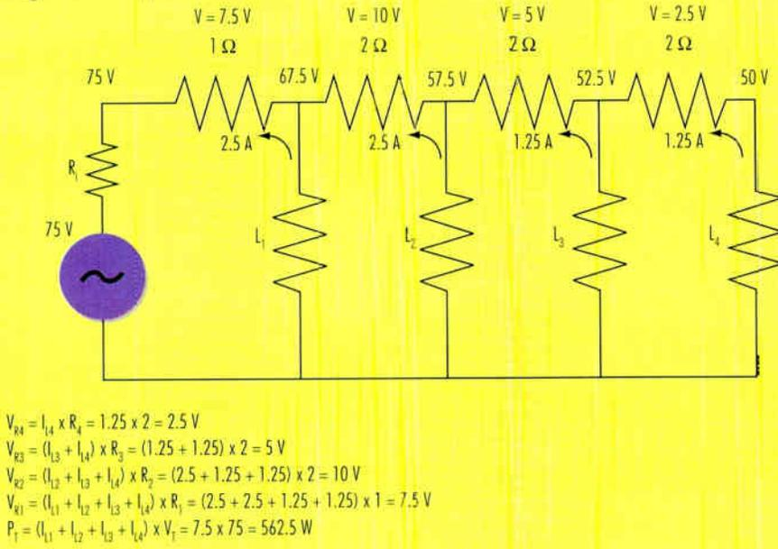
scriber, depending on the services provided and the population density of the area. This correlates to a power supply requirement of 400 W to 10,000 W; with 2,500 W very typical. A lot of power! Distance also becomes a concern due to the voltage loss of the distribution cable. Typical designs are limited to 6,000 to 7,000 feet. As power is carried along the cable, voltage is dropped across the cable's resistance, depending on the current in the cable.
