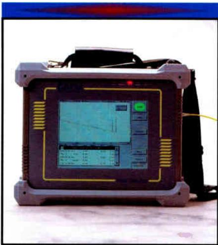
The purpose of the Optical Time Domain Reflectometer (OTDR) is to provide communications technicians and engineers the capability to analyze, test, and maintain a wide variety of fiber optic communications systems and equipment on the bench and in the field.
