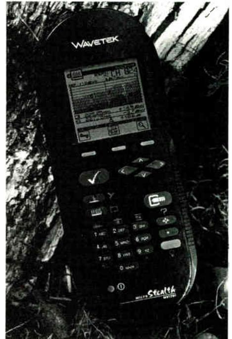
stallers. Both models have a durable, waterproof, high-resolution dot matrix LCD that provides ease of measurement with a scan display that shows multiple carrier levels at once and a comprehensive single-channel display.
