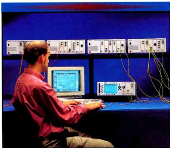
Years of research and study have resulted in the development of EXFO's new IQ-200 test instrument product family. The IQ-200 is a modular test system comprised of mainframes and modules, including high performance, programmable optical power meters, light sources, programmable variable attenuators, variable backreflectors, ORL testers, optical multimeters with remote heads, EDFAs, DFB lasers and optical switches, among many others.
