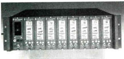
Using NAM550 frequency agile modulators, the Stratum Series will accept and combine a variety of audio, video and IF inputs, providing optimum rebroadcasting quality and spurious-free RF performance from 54-550 MHz.
