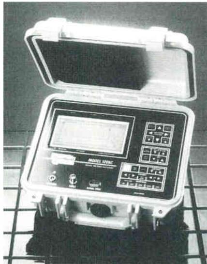
A unique function of the IFD feature is that the waveform can be manipulated, repositioned, zoomed in or out and the cursors moved — all without affecting the IFD function.
