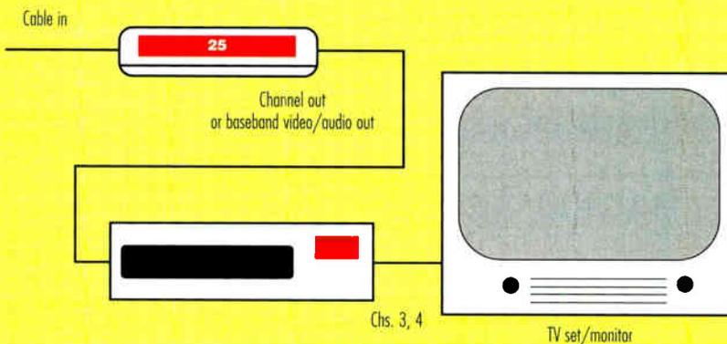
or monitor with either a baseband A/V signal or RF channel out to the RF input of the receiver. (See Figure 1.)
