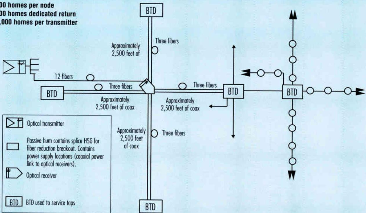
are opto-electronic and RF components, fiber, coaxial cable and power supplies. Excluded are headend electronics, set-top units and installation costs. Note that in lower density applications, the price per mile for 2,000 homes per node (HPN) vs. 500 HPN is relatively level. Therefore, density dictates the maximum attainable node size in this instance.
