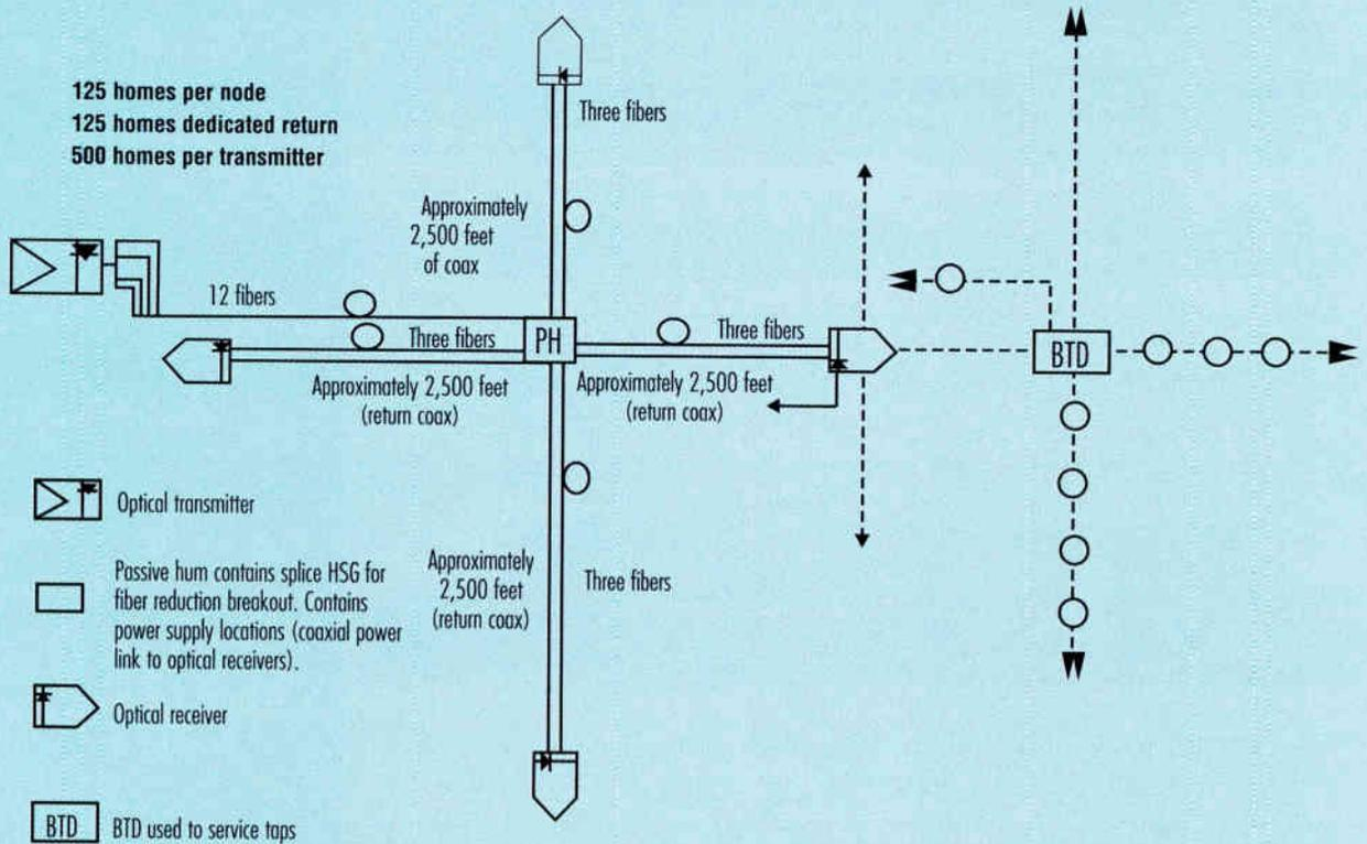
utilize higher power lasers (optically split to feed several nodes or lower power lasers for a point-to-point configuration). Note that the 500-home initial node is segmented, ideally into four smaller cells containing 125 homes each. This segmentation often depends upon system density and geography. Each segment then uses express (untapped) cable to the first active device in cascade and beyond if necessary.
