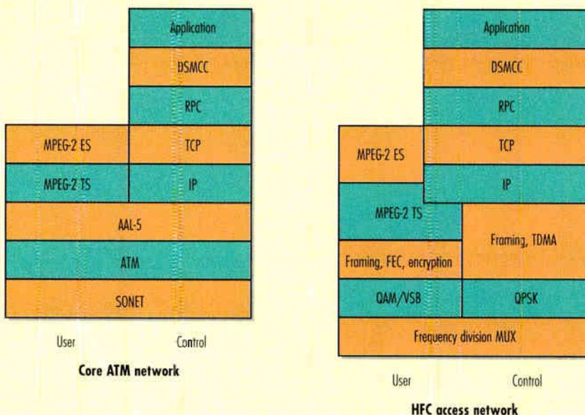
low for ATM signaling (Q.2931) by the set-top, however the digital storage media command and control (DSMCC) protocol allows the set-top to make session requests to the network. (This protocol is designated by the MPEG-2 DSMCC Working Group under the auspices of the International Standards Organization.)
