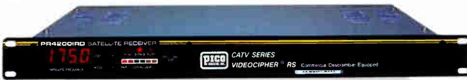
The PR4200IRD is an economic, micro-processor controlled commercial grade satellite receiver designed for CATV and SMATV systems. The receiver employs a phase locked loop demodulator to
