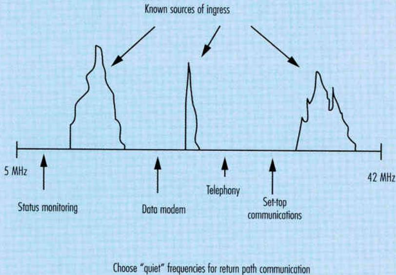
**Figure 4:** Carrier frequencies and guardbands
