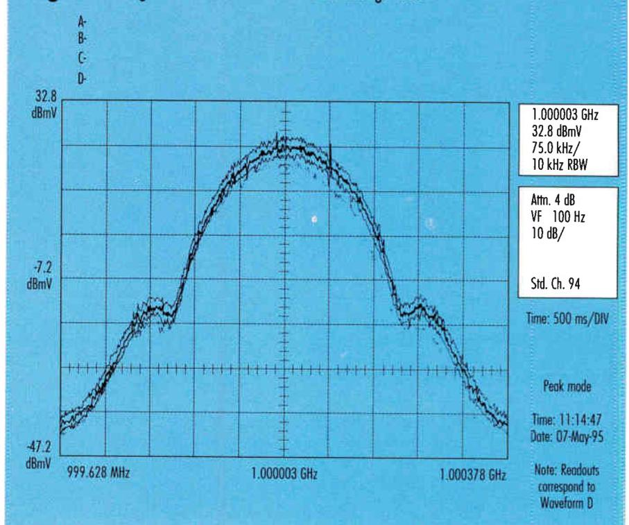
cally 54 dBmV. When all the calculations and performance measures are taken into account, we find that the dynamic range for both analog and digital, or mixed hybrid, signals is about 60 to 70 dB, depending on the number of carriers involved. This can lead to marginal results, which may require the use of an external input preselector to reduce the input signal loading.
