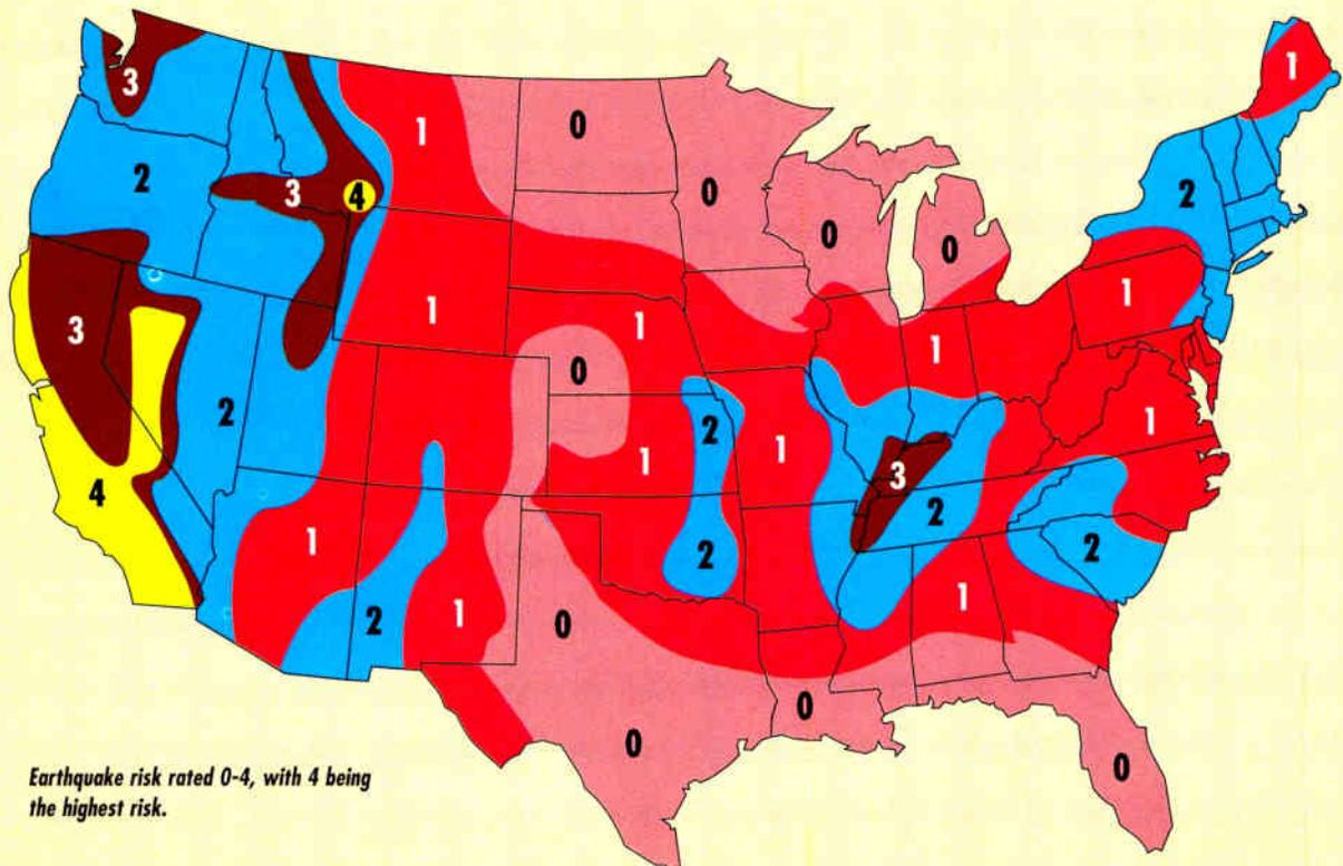
core. Bellcore publishes various technical references that are available to the industry for a small charge. The technical reference that applies to seismic activity and other vibration is TR-NWT 000063. This technical reference not only provides risk assessment for earthquake damage in the U.S. by geographic area, but also provides detailed setup inspections on how to test equipment for resistance to seismic activity.
