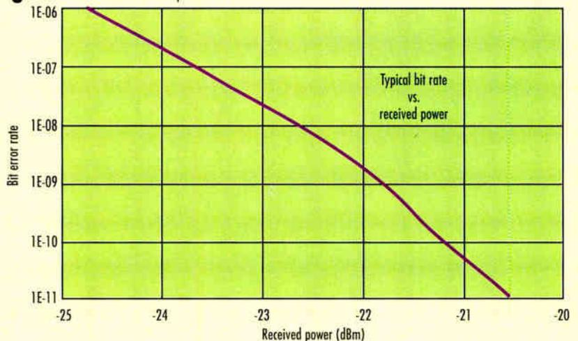
Bit error rate increases rapidly with drop in Rx power beyond minimum threshold.
