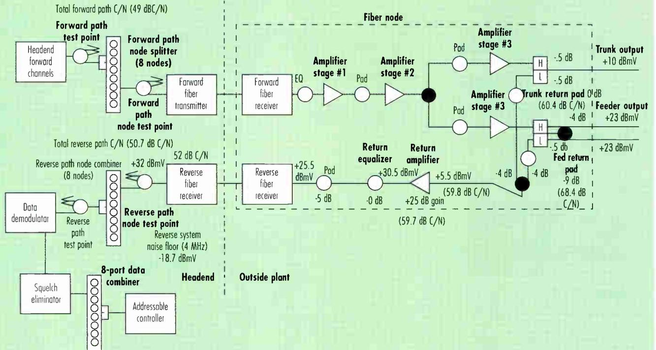
the outputs of the amplifiers are increased to the design limit of CTB, CSO and XMOD. This is done to ob-
