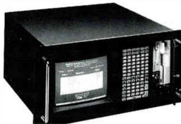
fully programmable digital controller automatically activates virtually any pay-per-view promo or video event, RF/IF modulator, satellite receiver, VTR and any other externally switched device in the headend.
